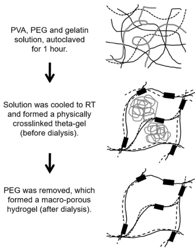
**Figure 1.** Schematic illustrating the formation of a PVA and gelatin theta-gel, through the physical crosslinking of PVA (solid black lines) and gelatin (dashed black lines), respectively, in the presence and subsequent removal of PEG. Areas of hydrogen bonding (i.e., physical crosslinks) between gelatin and PVA are represented by black rectangles. Nucleation of PEG porogens (gray lines) during solidification and subsequent removal through dialysis resulted in a macro-porous network.
