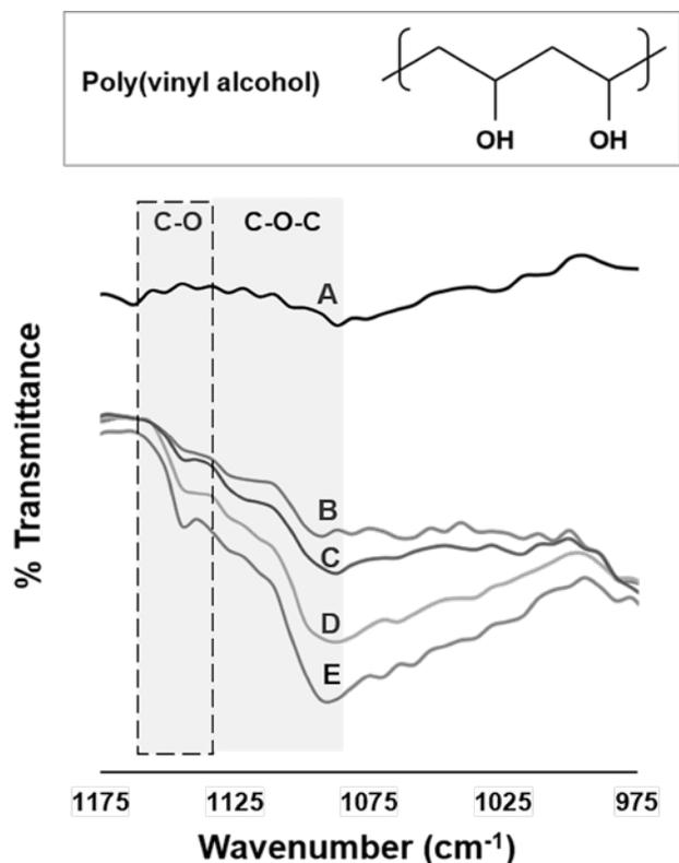
**Figure 2. Top:** Chemical structure of PVA; physical crosslinking takes place at OH groups between PVA molecules. *Bottom:* FTIR spectra of (A) gelatin, (B) PVA-PEG-1Gel, (C) PVA-PEG, (D) PVA-1Gel and (E) PVA hydrogel films. C-O stretching vibrational bands, associated with PVA physical crosslinking and crystallization, are shown. Samples were characterized after the removal of PEG porogens; PEG is incorporated into the group names to indicate the fabrication method.
