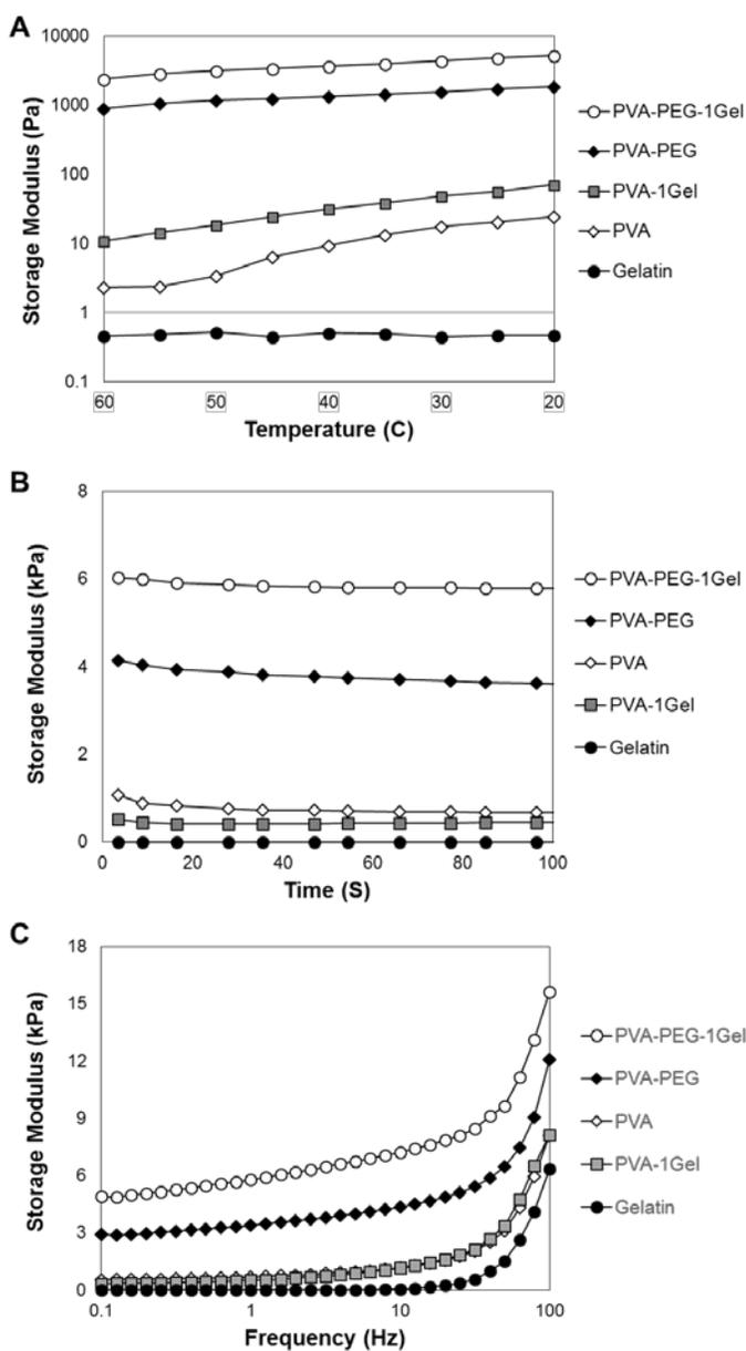
**Figure 4.** Rheological experiments were performed to examine the effect of PEG porogens during the solification of PVA-based hydrogels on the mechanical properties. A) Temperature sweeps of single macromers, control solutions (PVA-1Gel, PVA-PEG), and experimental solutions (PVA-PEG-1Gel) were tested from 60 °C to 20 °C to illustrate the gelation process of each sample. B) Oscillatory time sweep experiments for control hydrogels (gelatin, PVA, PVA-
