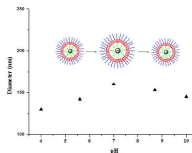
**Figure 7.** pH-dependent size of the micelles formed by the hybrid copolymer POSS-(PAA-(PLLA-OH)<sub>4</sub>)<sub>8</sub>.
