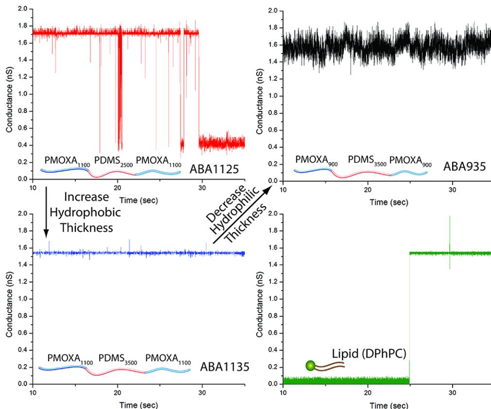
Figure 4. Conductance traces over 20 seconds with an applied voltage of 60mV for a single MspA insertion into ABA1125 (top left), ABA1135 (bottom left), ABA935 (top right) and DPhPC (lipid) (bottom right). All traces filtered with 10th-order Butterworth filter at 100 Hz.
