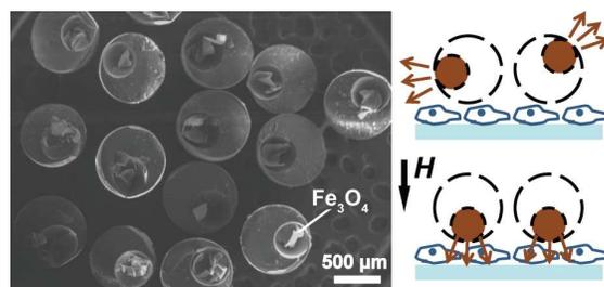
Uniform eccentric magnetic microcapsules show controlled-release behavior for orientation-specific and dual stimuli-responsive drug delivery under ultrasound and laser regulation.
