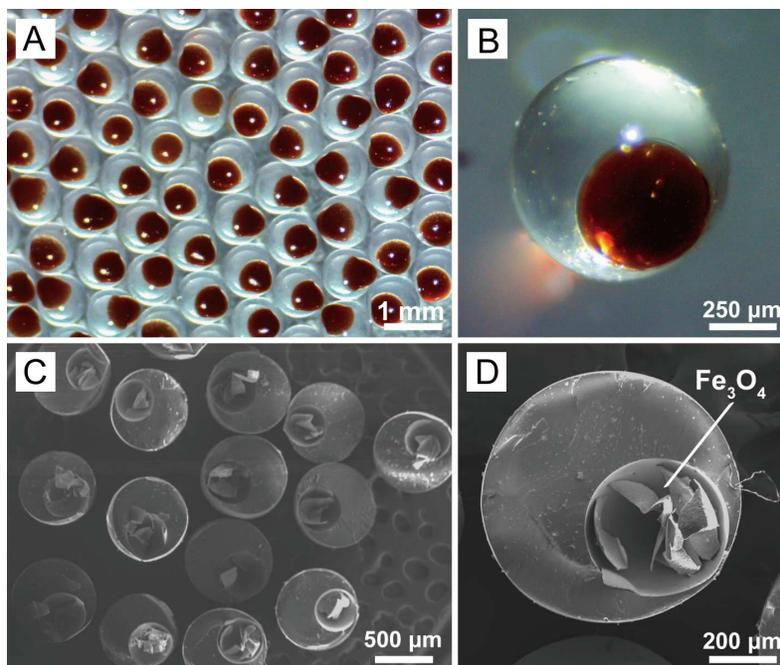
**Figure 1.** Observation of eccentric magnetic microcapsules. (A, B) Optical images of eccentric magnetic microcapsules. The inner aqueous phase contained magnetic nanoparticles. (C, D) Scanning electron microscope (SEM) images of eccentric magnetic microcapsules. The internal space contained magnetic nanoparticles which were dried after baking for imaging.
