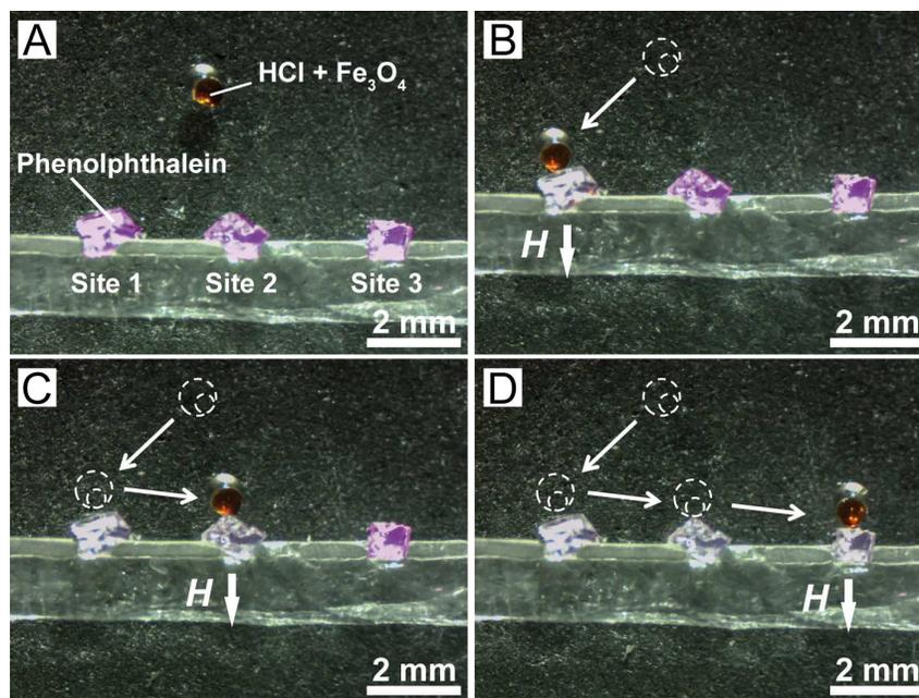
**Figure 2.** Site-specific control of one eccentric magnetic microcapsule under magnetic field. (A) Optical image of an eccentric magnetic microcapsule and a PDMS receptacle with three targets at different sites. (B, C, and D) Optical images showing the process of site-specific control of the microcapsule. Microcapsule was moved and located to the three target sites sequentially under the attraction of a small magnet.
