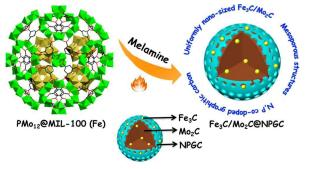
Scheme 1 Preparation of  ${\rm Fe_3C/Mo_2C@NPGC}$  nanocomposite derived from POM-based MOFs.
