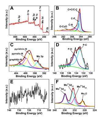
Fig. 2 XPS survey spectra (A) and high-resolution scans of (B) C 1s, (C) N 1s, (D) P 2p, (E) Fe 2p, and (F) Mo 3d electrons of Fe<sub>3</sub>C/Mo<sub>2</sub>C@NPGC.
