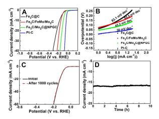
Fig. 3 (A) Polarization curves of different samples. (B) Corresponding Tafel plots of the polarization curves. (C) Polarization curves of  $Fe_3C/Mo_2C@NPGC$  initially and after 1000 cycles. (D) Time dependence of current density under static overpotential of 120 mV for 10 h.
