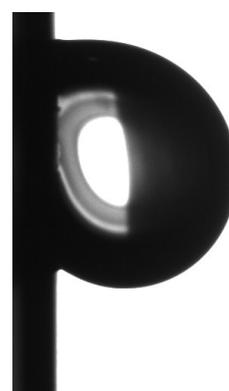
**Fig. 2** Picture of a water droplet put on PolyNaphDOT, obtained by cyclic voltammetry (3 scans), and after a surface inclination of  $90^\circ$ .
