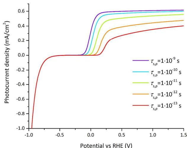
**Figure 8** Photocurrent-voltage curves for varying hole surface lifetimes for the reference case (parameters indicated in Table 1 and 2). For large hole surface lifetimes (above 0.1 to 1 ns), surface recombination is negligible at large applied potentials. For small hole surface lifetimes (around 1 ps), the photocurrent is still affected by surface recombination at large potentials.
