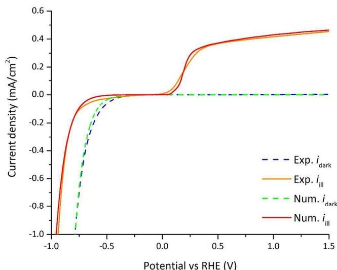
**Figure 6** Dark current densities (dashed lines) and photocurrent densities (solid lines) vs RHE, and comparison between experimentally measured values and numerically calculated values.
