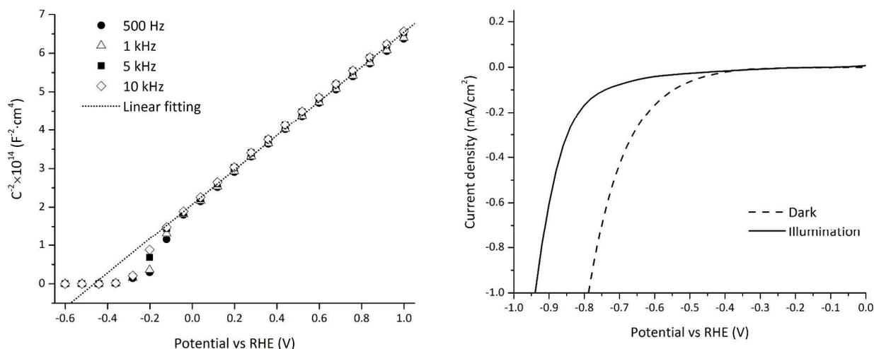
**Figure 5 a) Mott-Schottky plot for four frequencies (500 Hz, 1 kHz, 5 kHz, 10 kHz) of a 1  $\mu$ m-thick n-doped GaN sample immersed in 1M  $H_2SO_4$  electrolyte under dark. b) Experimental dark current density (dashed line) and photocurrent density (solid line) vs RHE.**
