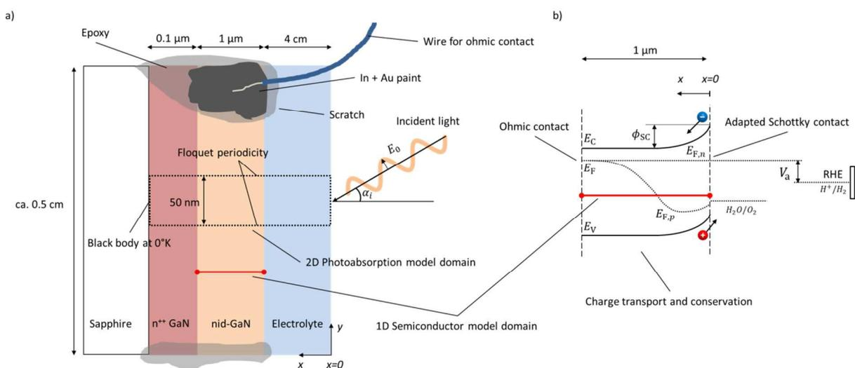
**Figure 1** a) Scheme of the model domain (not to scale) of the photoanode (GaN) immersed in electrolyte including the 2D EMW propagation model domain (dotted) and boundary conditions, and the 1D semiconductor model domain (red line). b) Detailed 1D semiconductor model domain and boundary conditions.  $E_C$  and  $E_V$  are
