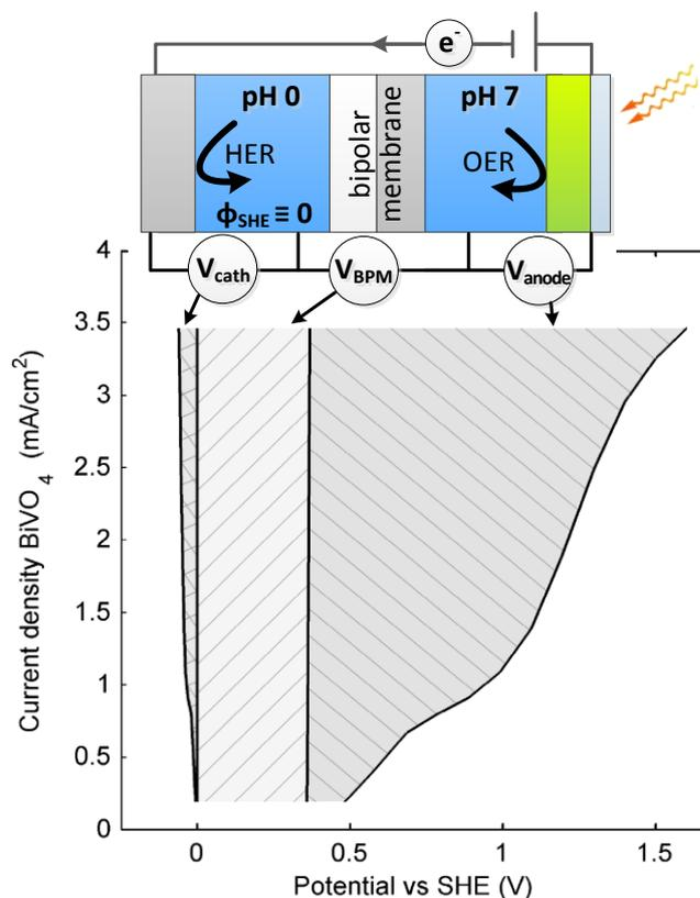
Figure 3: Potential differences over the cathode ( $V_{\text{cath}}$ ), over the bipolar membrane ( $V_{\text{BPM}}$ ) and over the anode ( $V_{\text{anode}}$ ), obtained in the same configuration as for Fig. 2, except that the anode operates in pH 7 in this case. No correction for ohmic losses is applied.
