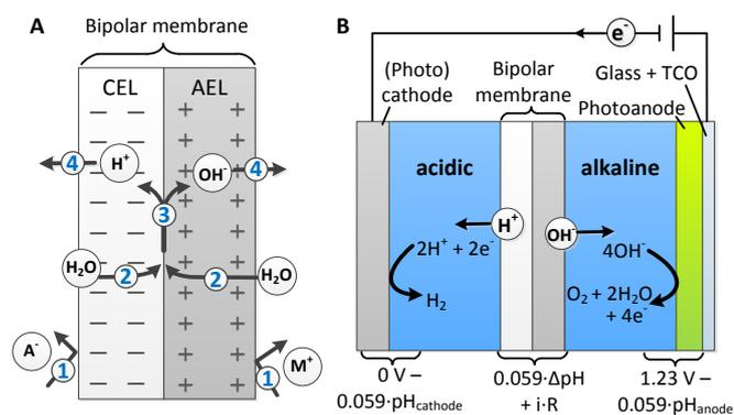
Figure 1. A: Working principle of a bipolar membrane. Positive ions ( $M^+$ ) cannot enter the anion exchange layer (AEL) and negative ions ( $A^-$ ) cannot enter the cation exchange layer (CEL) (1). This results in water dissociation on the interface of these two layers (3), which is supplied by water diffusion (2) and leads to transport of  $H^+$  and  $OH^-$  (4). B: an example of a bipolar membrane implemented in a solar fuel system, with 1 or possibly 2 photoelectrodes.
