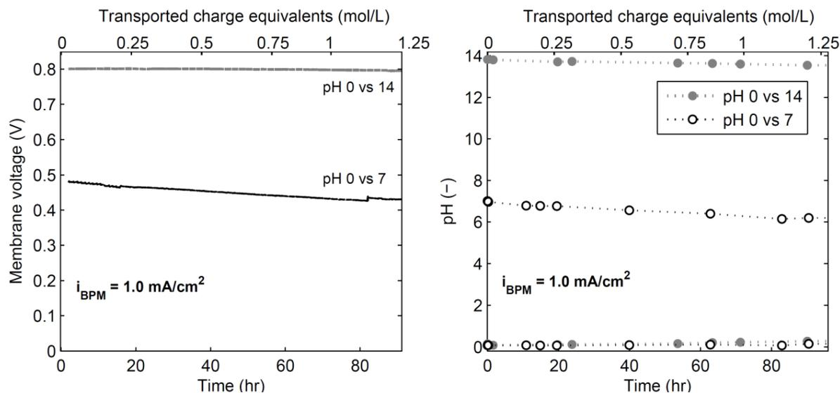
Figure 5: Membrane voltage (left) and pH (right) as a function of time, at a constant current density of  $1 \text{ mA/cm}^2$  of BPM area (which corresponds to  $12.8 \text{ mA/cm}^2$  anode area in this case). Inert (Pt) electrodes were used as anode and cathode in this case.
