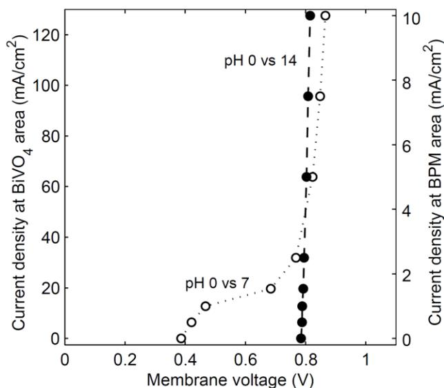
Figure 4: voltage over the bipolar membrane using a pH difference of 0-7 and 0-14 over the membrane as a function of the current density. The potentials were averaged over at least 300 s of constant current. As the bipolar membrane (BPM) area was larger than the BiVO<sub>4</sub> area, the corresponding current density for BiVO<sub>4</sub> is plotted as a secondary x-axis. No correction for ohmic losses is applied.
