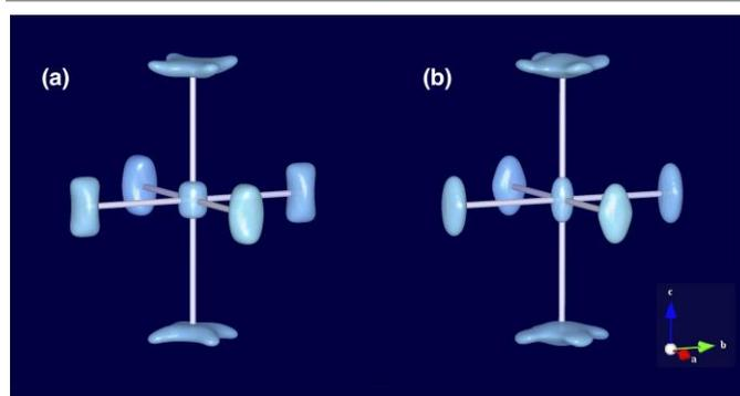
**Fig. 2:** Representation of the NiO<sub>6</sub> octahedra in NNO (a) and PNO (b) obtained from Maximum Entropy reconstruction of single crystal neutron diffraction data (5C2@LLB, ORPHEE reactor Saclay) at room temperature. Equatorial and apical oxygen atoms are strongly disordered showing huge anisotropic displacement parameters. The isosurfaces of the apical oxygen atoms evidence libration modes along the [110] direction of the *F*-centred unit cell, modes that appear to be sharper for NNO.
