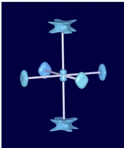
**Fig. 4:** Representation of the isosurfaces of the NiO<sub>6</sub> octahedron in Pr<sub>2</sub>NiO<sub>4.25</sub>, obtained from Maximum Entropy reconstruction of single crystal neutron diffraction data at 400°C (HEiDi@MLZ, FRM II reactor in Garching).
