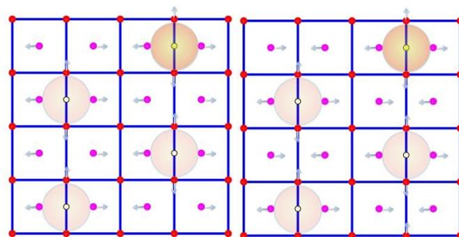
Fig. 6: Possible apical oxygen shift scenarios, taking into account an exact stoichiometry of PNO. Apical oxygen atoms of different heights (red:  $z = 0.17$ ; magenta:  $z = 0.33$ ) are indicated for one rock-salt type layer; a big yellow/reddish circle shows steric influence of the interstitial atoms, displacements indicated by arrows. A  $4 \times 4$  I4/mmm unit cell is outlined in blue, the arrows pointing towards the [110] direction of the F-cell.
