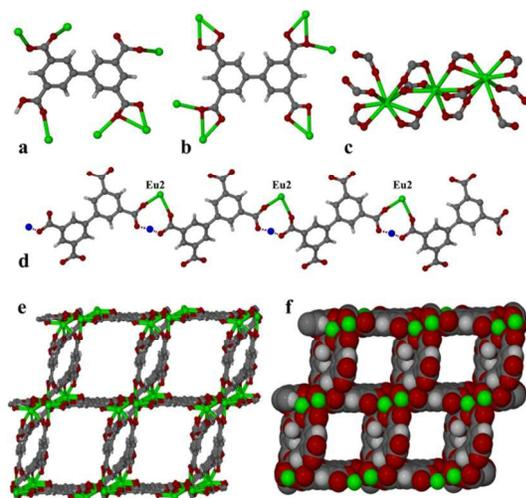
**Fig. 1** The coordination modes of <sup>a</sup>BPTC (a), <sup>b</sup>BPTC (b); the trinuclear “hourglass” SBU (c); the 1D supramolecular chain (d); the 3D porous framework with 1D channel along b axis (e), and space-filling representation
