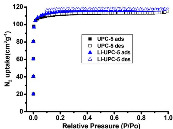
Fig. 2  $N_2$  adsorption isotherms for UPC-5 and Li-UPC-5.
