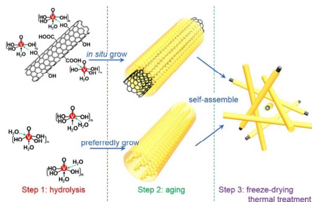
Fig. 1 Illustration of the mixed growth and self-assembly methodology for controlled synthesis of 3D V 2 O 5 /MWCNTs core/shell hybrid aerogels.
