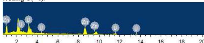
**Fig. 9** EDS spectra of the as-synthesized samples after loading U(VI).
