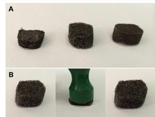
**Fig. 10** Photographs of G-Gel deposited on various sponges (A), and compressibility of the G-Gel deposited sponge (B).
