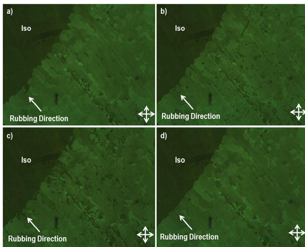
**Figure 17:** Domains observed (x100) upon annealing the higher temperature phase of **M10** (9.8 wt%) at  $81.5^\circ\text{C}$ : a) no field, b) immediately after application of 33 Hz,  $12 \text{ V } \mu\text{m}^{-1}$  sq. waveform field, c) immediately upon removal of field, and d) 5 minutes after removal of field.
