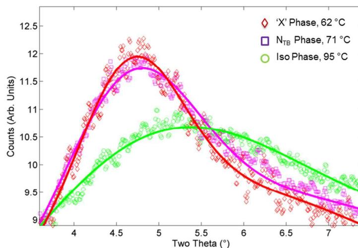
**Figure 14:** Plot of counts (arbitrary units) vs. two theta (°) for M10 in the lower isotropic (95 °C), N<sub>TB</sub> (71 °C) and "X" (62 °C) phases. Solid lines are fitted to the data using a 6-term Gaussian distribution. All fits give an R<sup>2</sup> value in excess of 0.99.
