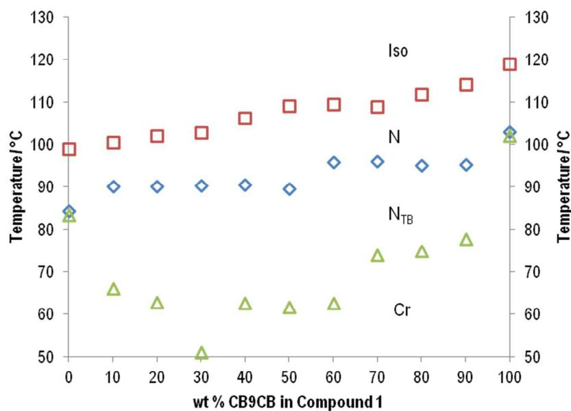
**Figure 4:** Gibbs phase diagram for binary mixtures (wt%) of compound 1 with CB9CB.
