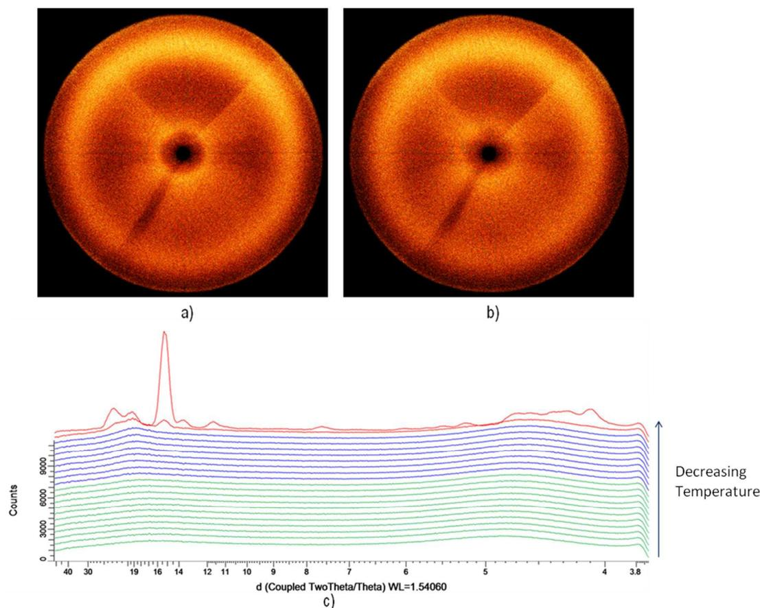
**Figure 12:** Two dimensional X-ray diffraction patterns obtained for mixture **M10** (9.8 wt% of compound **2** at; a) 71 °C in the  $N_{TB}$  phase, and b) 95 °C in the "isotropic" phase. c) A plot of d spacing as a function of temperature with measurements taken every 3 °C from 116 °C – 54 °C.
