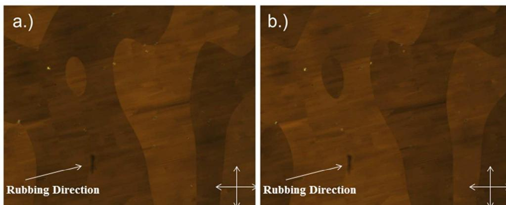
**Figure 15:** Evidence of opposite switching in the domains of the  $N_{TB}$  phase upon application of an electric field. Polarised optical microscope image of **1** in a  $5\ \mu\text{m}$  cell with an antiparallel buffed polyimide alignment layer subjected to an electric field (1 Hz,  $20\ \text{V}\ \mu\text{m}^{-1}$ , square waveform) at  $81\ ^\circ\text{C}$ . (x100)
