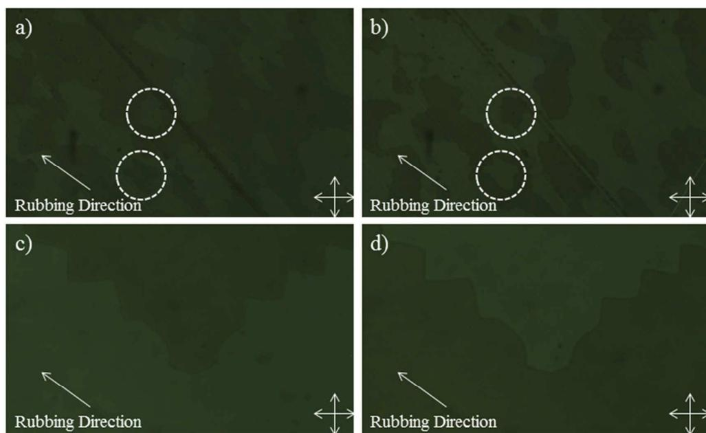
**Figure 16:** Evidence of opposite switching in the domains of the "platelet" phase upon application of an electric field. Polarised optical microscope images of **M10** (9.8 wt%) (x100) in a  $5\ \mu\text{m}$  cell with an antiparallel buffed polyimide alignment layer and subjected to an electric field (1 Hz,  $12\ \text{V}\ \mu\text{m}^{-1}$ , square waveform) at  $81\ ^\circ\text{C}$  (a and b) and  $81.5\ ^\circ\text{C}$  (c and d)
