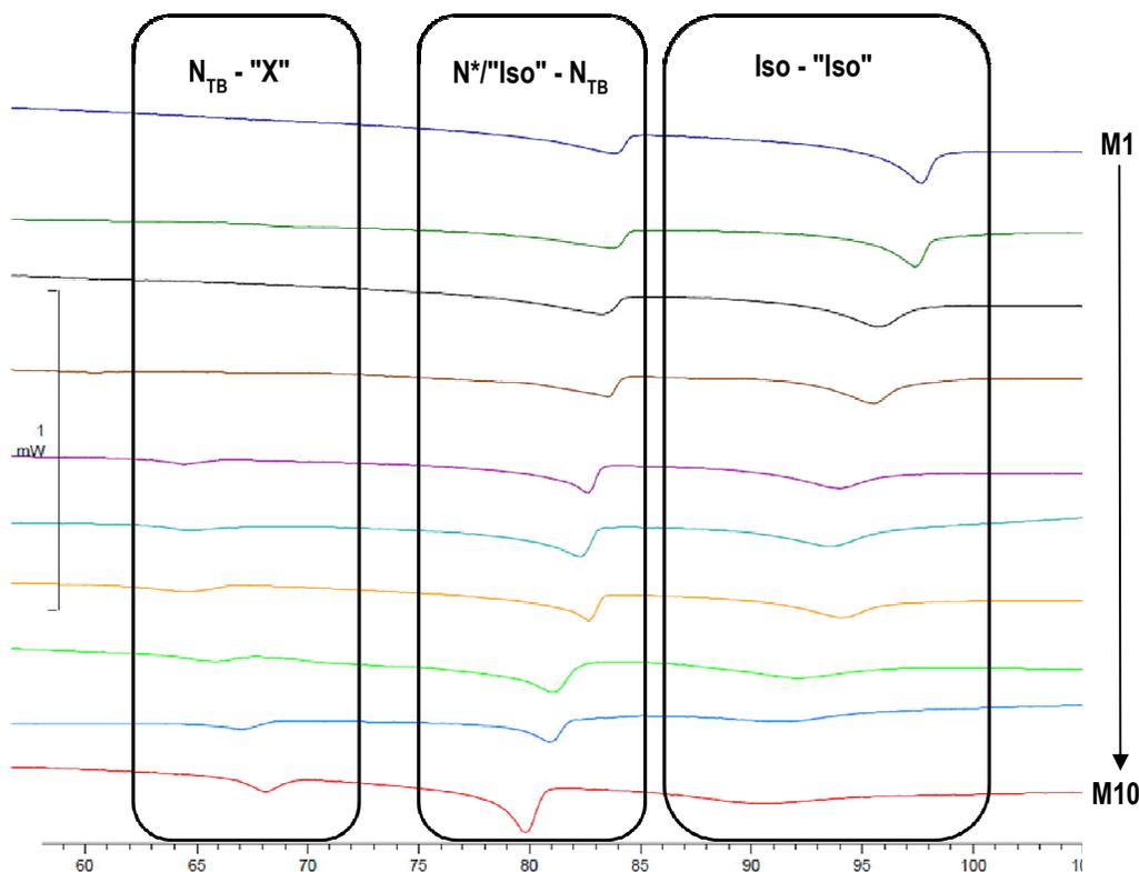
**Figure 9:** Plot of DSC traces (heat flow [mW] vs. temperature [°C],  $10\text{ }^{\circ}\text{Cmin}^{-1}$ ) on cooling for varying concentrations of compound 2 in compound 1.
