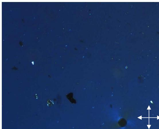
**Figure 6:** Photomicrograph showing the BPlll texture of mixture **M3** (5.4 wt %) at 93 °C. Sample was cooled at 0.1 °C min<sup>-1</sup> (x100).
