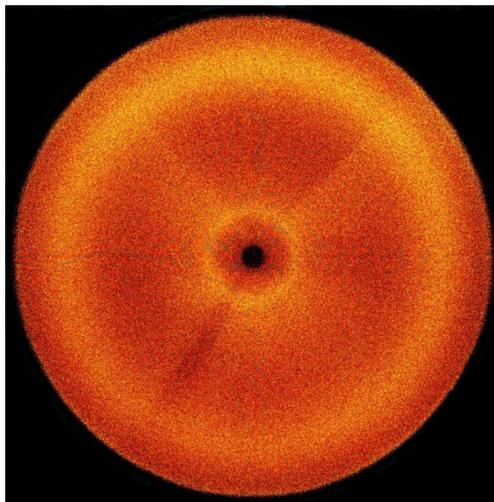
**Figure 13:** 2D XRD pattern of mixture **M10** (9.8 wt%) in the lower temperature "X" phase (62 °C).
