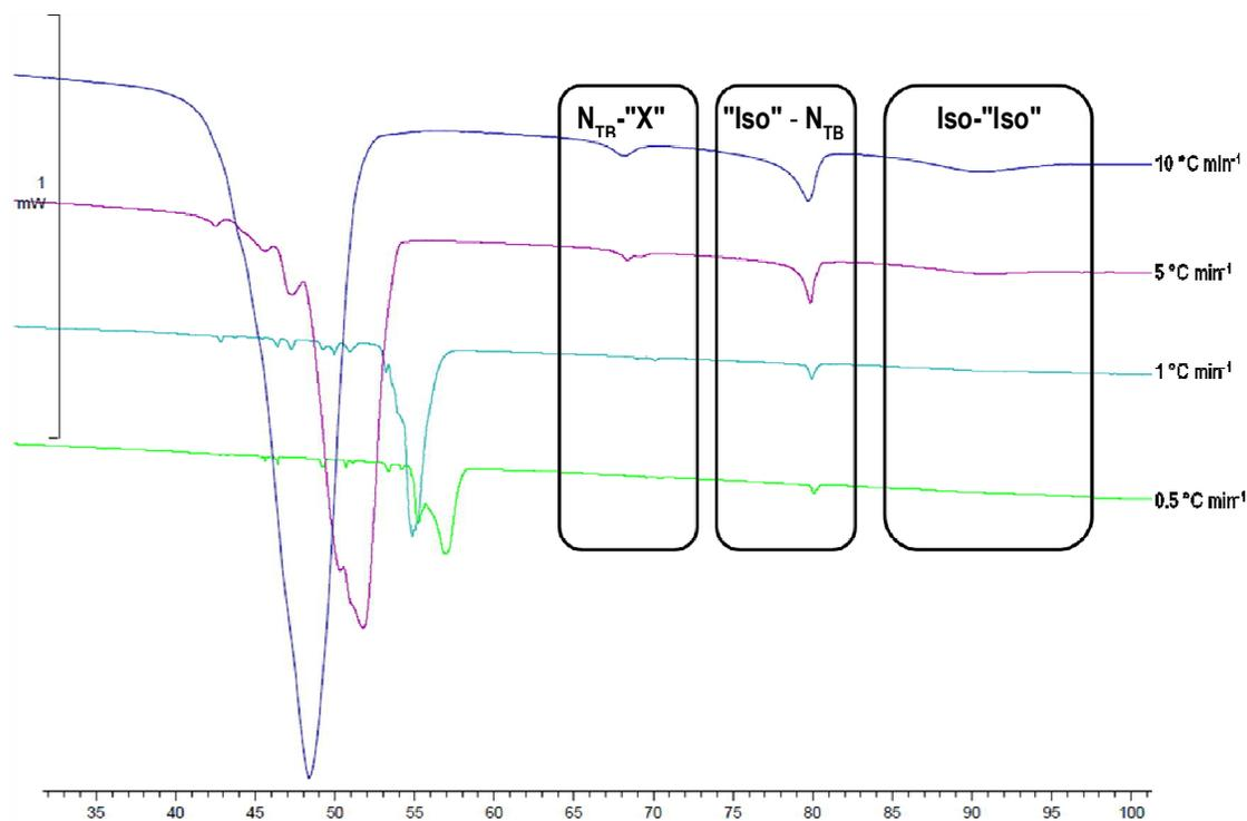
**Figure 10:** Plot of DSC traces (heat flow [mW] vs. temperature [°C],  $10^{\circ}\text{Cmin}^{-1}$ ) on cooling for mixture **M10** at various cooling rates.
