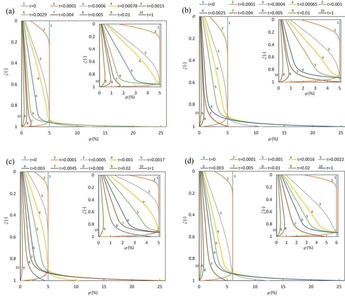
**Fig. 4.** Time evolution of liquid volume fraction over the foam height at a)  $Bo=9.81$ ,  $\alpha=10$ ,  $\varepsilon=0.03$  and  $\varphi(z, 0)=5\%$ ; b)  $Bo=5.45$ ,  $\alpha=25$ ,  $\varepsilon=0.03$  and  $\varphi(z, 0)=5\%$ ; c)  $Bo=5.45$ ,  $\alpha=10$ ,  $\varepsilon=0.02$  and  $\varphi(z, 0)=5\%$ ; d)  $Bo=5.45$ ,  $\alpha=10$ ,  $\varepsilon=0.03$  and  $\varphi(z, 0)=6\%$ . In all cases inserts present enlarged region of liquid content from 0 to 5-6%.
