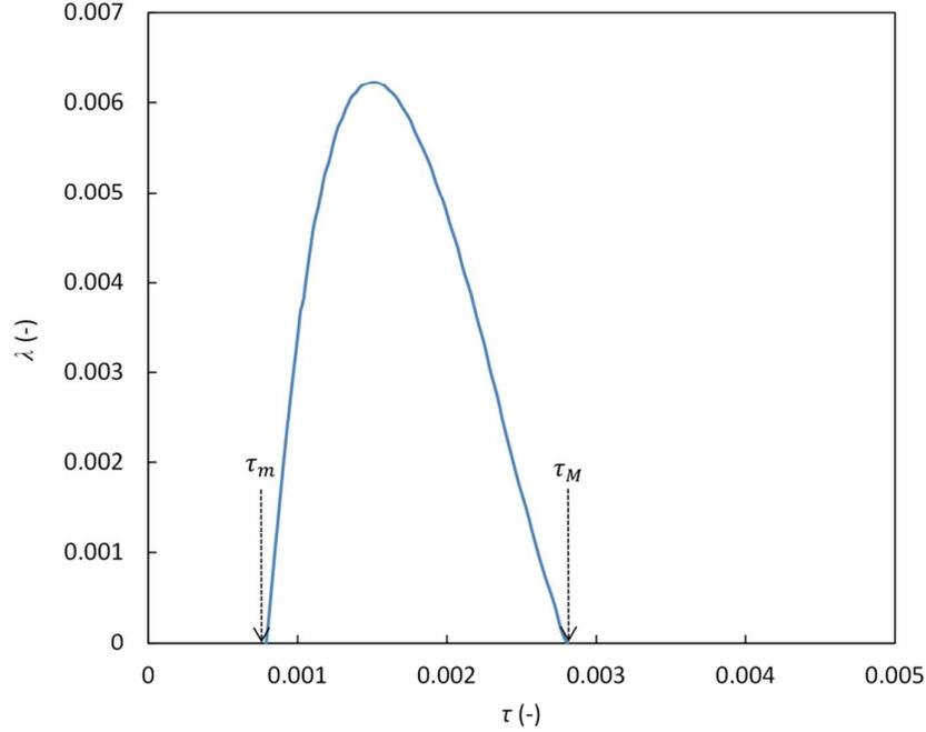
**Fig. 5.** Time evolution of the thickness of free liquid layer between foam and porous substrate at  $Bo=9.81$ ,  $\alpha=10$ ,  $\varepsilon=0.03$  and  $\varphi(z, 0)=5\%$  (corresponds to Fig. 4(a)).
