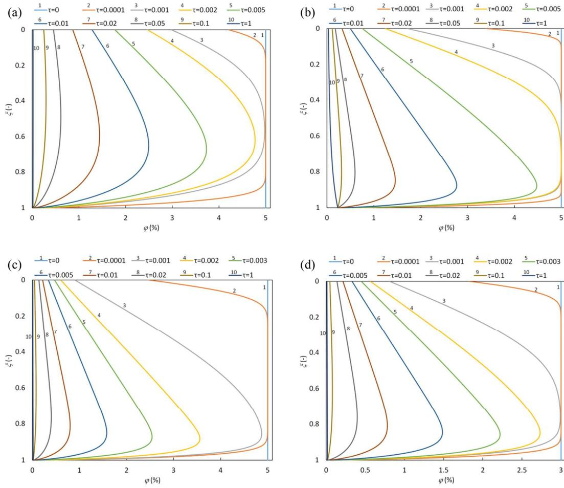
**Fig. 3.** Time evolution of liquid volume fraction over the foam height at a)  $Bo=1.23$ ,  $\alpha=10$ ,  $\varepsilon=0.03$  and  $\varphi(z, 0)=5\%$ ; b)  $Bo=5.45$ ,  $\alpha=2$ ,  $\varepsilon=0.03$  and  $\varphi(z, 0)=5\%$ ; c)  $Bo=5.45$ ,  $\alpha=10$ ,  $\varepsilon=0.06$  and  $\varphi(z, 0)=5\%$ ; d)  $Bo=5.45$ ,  $\alpha=10$ ,  $\varepsilon=0.03$  and  $\varphi(z, 0)=3\%$
