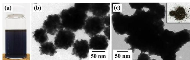
Figure 1. (a) Photographic and (b) TEM images of as-prepared Au NFs before the water extraction. (c) TEM and inserted photographic images of unsupported Au NFs after third extraction.
