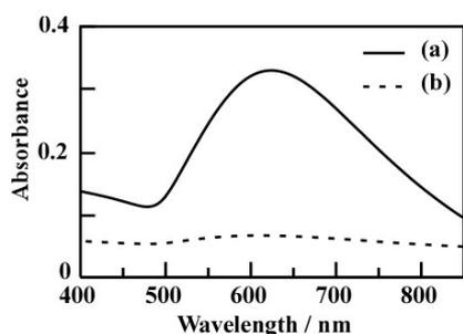
Figure 2. UV-vis absorption spectra of unsupported Au NFs (a) before the water extraction (solid line) and (b) after third extraction (dashed line).
