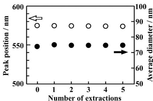
Figure 7. Peak positions of surface plasmon band (open circles) and average diameter (filled circles) of Au NFs on Al<sub>2</sub>O<sub>3</sub> before and after water extraction procedure.
