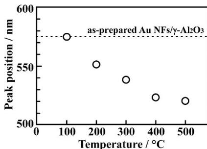
Figure 5. Peak position of SP band before and after calcination. Black dotted line is peak position of as-prepared Au NFs/ $\gamma$ -Al<sub>2</sub>O<sub>3</sub>.
