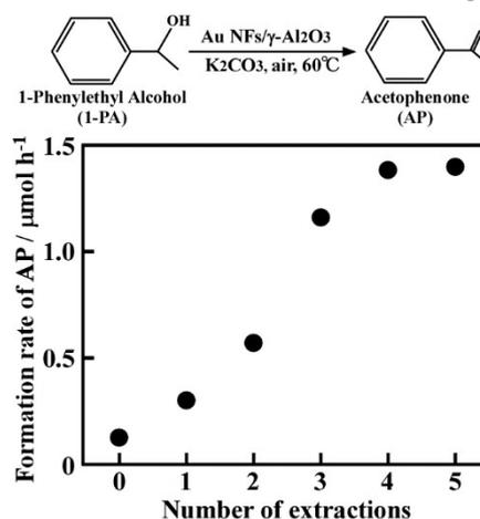
Figure 8. Change in formation rate of acetophenone at 6 h in 1-phenylethyl alcohol oxidation with number of repeated extractions.
