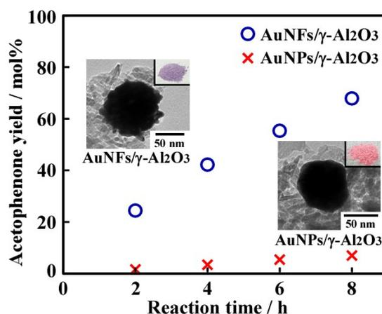
Figure 10. Acetophenone yield of *surface clean* Au NFs/ $\gamma$ - $\text{Al}_2\text{O}_3$  and Au NPs/ $\gamma$ - $\text{Al}_2\text{O}_3$ . Reaction conditions: 1-phenylethyl alcohol (15  $\mu\text{mol}$ ), catalyst (50 mg),  $\text{K}_2\text{CO}_3$  (0.1 g), water (10 g), air (1 atm), 60°C.
