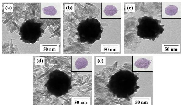
Figure 6. TEM and photographic images of Au NFs/ $\gamma$ -Al<sub>2</sub>O<sub>3</sub> after water extraction procedure carried out (a) one, (b) two, (c) three, (d) four, and (e) five times.
