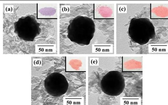
Figure 4. TEM and photographic images of Au NFs/ $\gamma$ - $\text{Al}_2\text{O}_3$  after calcination at (a)  $100^\circ\text{C}$ , (b)  $200^\circ\text{C}$ , (c)  $300^\circ\text{C}$ , (d)  $400^\circ\text{C}$ , and (e)  $500^\circ\text{C}$ .
