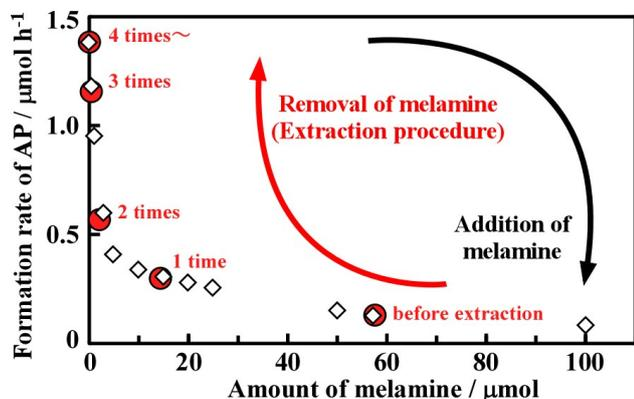
Figure 9. Change in the formation rate of acetophenone in 1-phenylethyl alcohol oxidation over Au NFs/ $\gamma$ - $\text{Al}_2\text{O}_3$  with amount of added (open squares) or residual (filled circles) melamine. Reaction conditions: 1-phenylethyl alcohol (15  $\mu\text{mol}$ ), catalyst (50 mg),  $\text{K}_2\text{CO}_3$  (0.1 g), water (10 g), air (1 atm), 60°C, 6 h.
