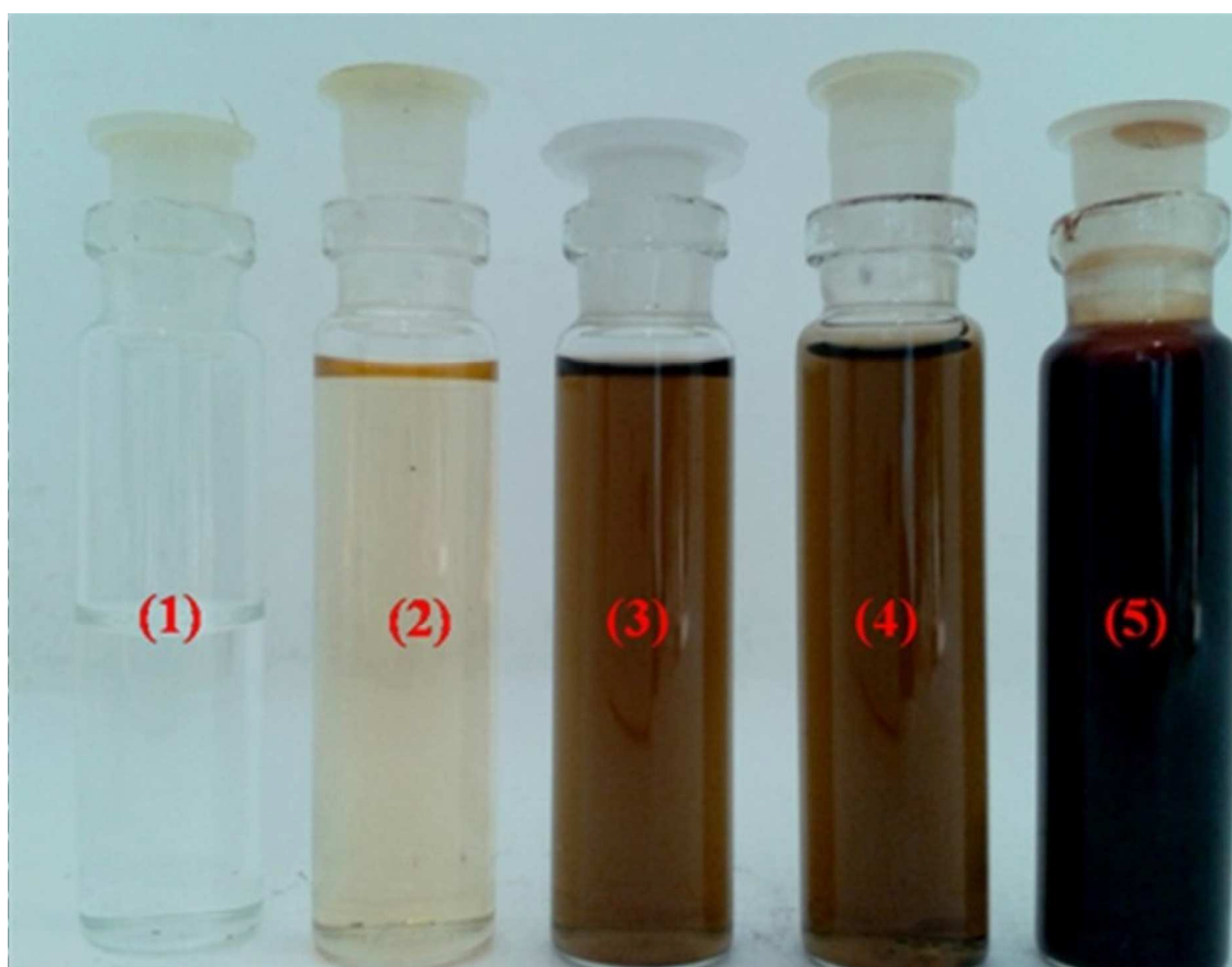
Figure 8. Photographs of phenol degradation process for (1) MC-1, (2) MC-5, (3) MC-10, (4) MC-15 and (5) CD-MC-15 catalysts, respectively
