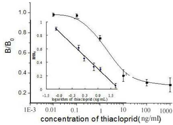
Fig.2 Calibration curve for thiacloprid by ECL-EIA
