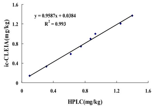
Fig. 3 Correlation between ECL-EIA and HPLC results for real tomato samples
