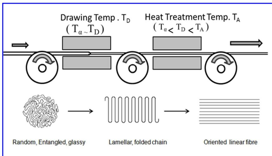
**Fig. 4** Schematic diagram of multi-stage steam drawing unit for fabrication of fine sized SAF ( $T_\alpha$ ,  $T_D$  &  $T_A$  refers to temperature of softening, drawing and annealing, respectively)
