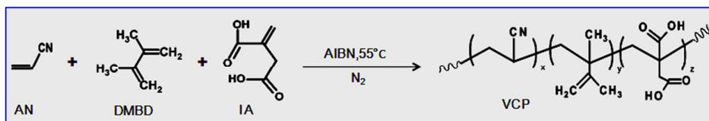
Scheme 2 PAN copolymerization reaction used in this study
