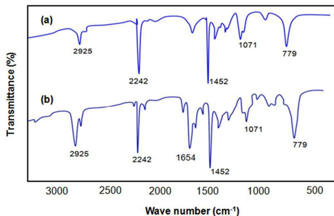
**Fig. 1** FTIR spectra of (a) VHP01 & (b) VCP02/03 polymers**Table 2** Principal IR bands in solid VHP and VCP01/02
