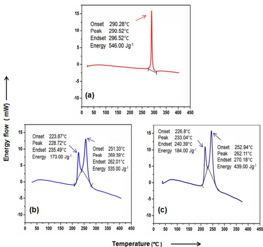
**Fig. 8** DSC exotherm of (a) VHP01 and (b & C) VCP 01/02 polymers in nitrogen
