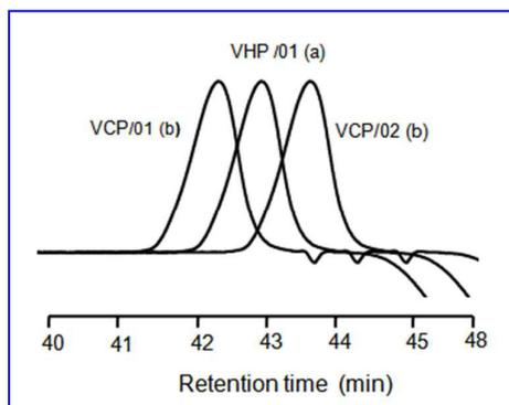
**Fig. 3** Traces of SEC-LALLS elution curves (a) VHP and (b) VCP polymers in dimethylformamide
