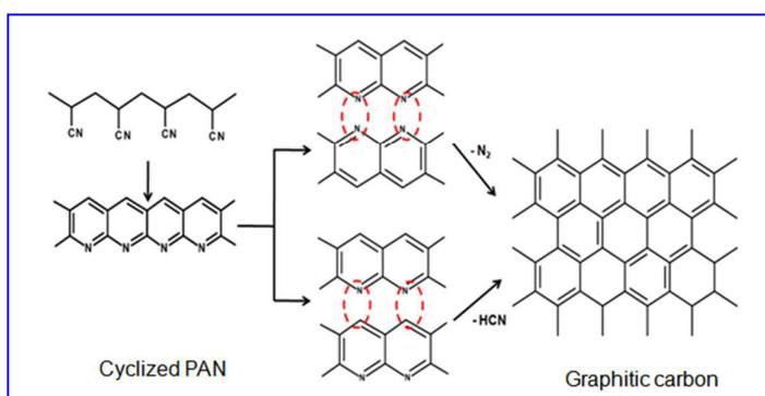
**Scheme 1** PAN polymer structure with pendant nitrile groups leading to graphitic structure
