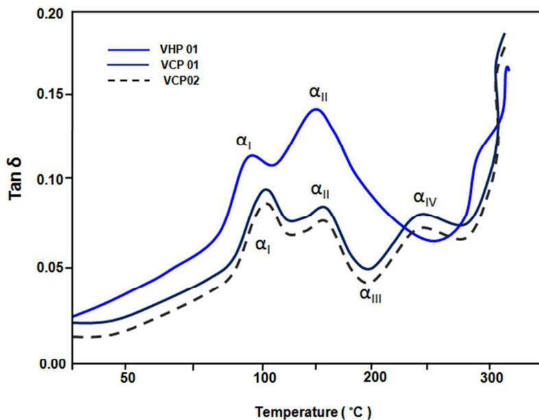
**Fig.5** Plots of  $\text{Tan } \delta$  versus temperature of the VCP 01/02 and VHP/01 polymers
