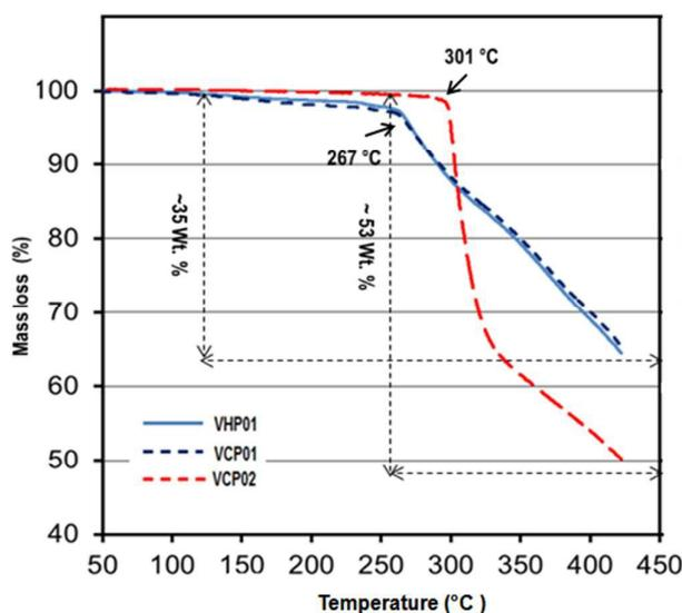
**Fig. 7** Thermogravimetric mass loss curves of VCP01/02 and VHP polymers.
