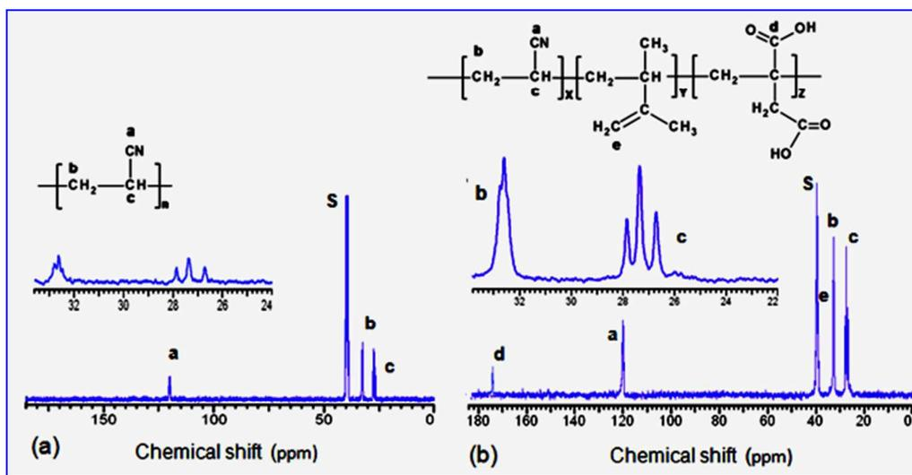
**Fig. 2**  $^{13}\text{C}$  NMR Spectra of (a) VHP and (b) VCP polymers in DMSO; Methine and methylene carbon region expanded.
