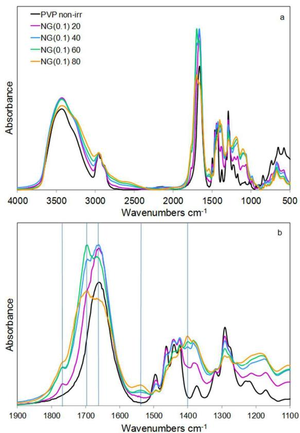
**Figure 7a-b.** FTIR spectra of NG(0.1) systems irradiated at various doses: (a) full spectra; (b) enlargement in the 1900-1100  $\text{cm}^{-1}$  wavenumbers range.
