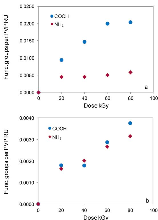
**Figure 9a-b.** Number of carboxyl and primary amino groups formed on PVP nanogels irradiated at 0.1 wt% (a) and 0.5 wt% (b) as function of the irradiation dose
