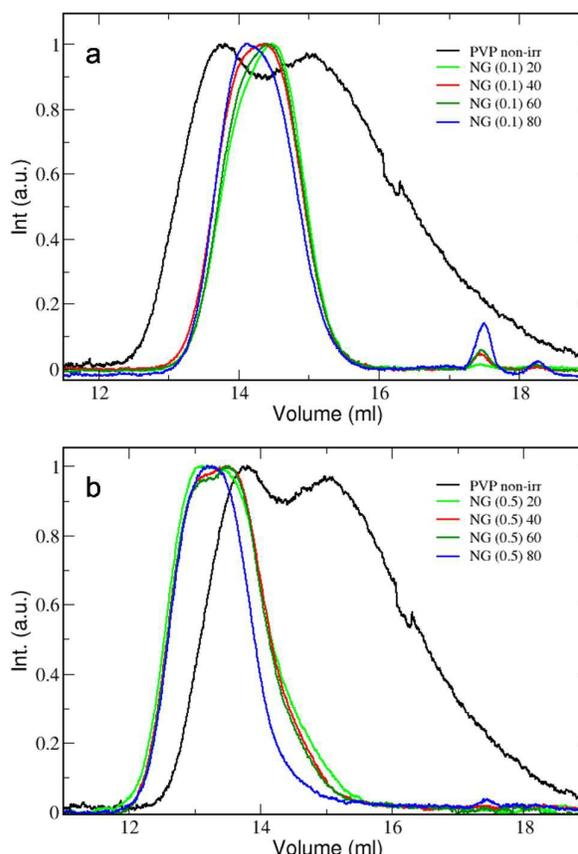
**Figure 5a-b.** Chromatographic profiles for the nanogels produced at 0.1 % wt (a) and 0.5 % wt (b), varying the total dose. The GFC curve for the non-irradiated polymer is also included as reference.
