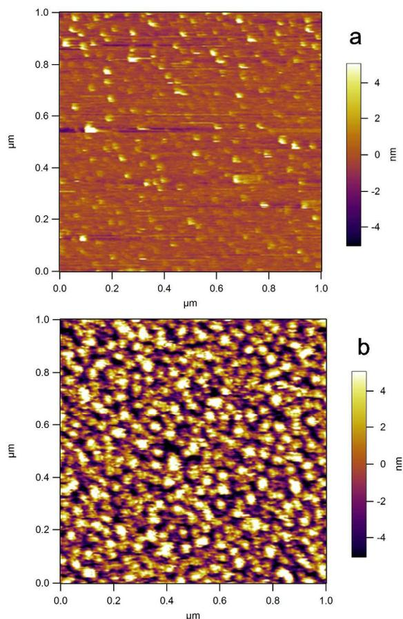
**Figure 6a-b.** Height profiles from tapping mode AFM under water show for the NG(0.1) 40, (a), and NG(0.5) 40, (b). The color scale represents a maximum height of 8 nm.
