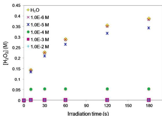
**Figure 2.**  $\text{H}_2\text{O}_2$  concentrations as function of irradiation time for pure water and for aqueous solutions containing various concentrations of hydroxyl radical scavengers during continuous irradiation at the dose rate during the pulse ( $16 \text{ MGy s}^{-1}$ ). Results obtained from numerical simulations.
