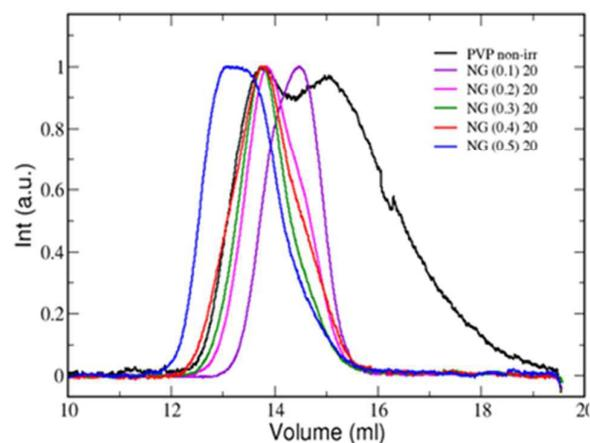
**Figure 4.** Chromatographic profiles for the nanogels produced at 20 kGy, varying the polymer concentration. The GFC curve for the non-irradiated polymer is also included as reference.
