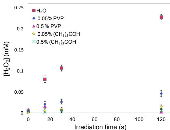
**Figure 3.**  $\text{H}_2\text{O}_2$  concentration as a function of irradiation time at a pulse length of 50 ns and a frequency of 25 Hz for  $\text{N}_2\text{O}$  saturated water and aqueous solutions containing PVP and  $(\text{CH}_3)_3\text{COH}$
