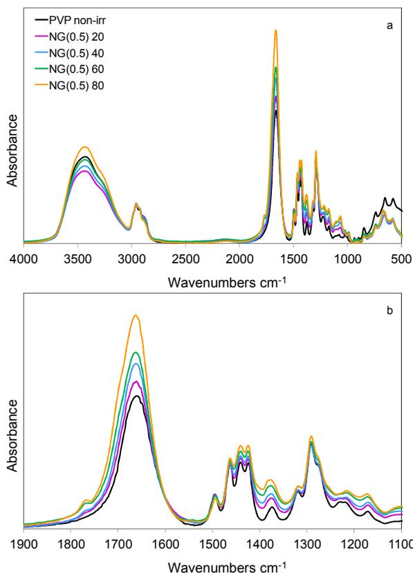
**Figure 8a-b.** FTIR spectra of NG(0.5) systems irradiated at various doses: (a) full spectra; (b) enlargement in the 1900-1100  $\text{cm}^{-1}$  wavenumbers range.
