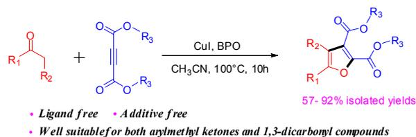
**Scheme 1.** Synthesis of furan from ketone and alkynoate.
