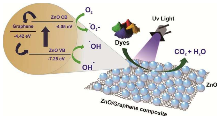
Fig. 11 Schematic diagram of proposed mechanism for the photodegradation of dyes over the ZnO/Gr nanocomposite under UV light.
