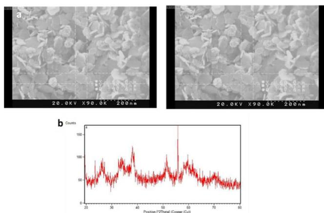
**Figure 1.** a: FE-SEM images and b: XRD patterns of cobalt oxid nanoparticles
