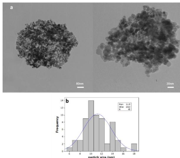
**Figure 2.** a: TEM images and b: particle size distribution results for cobalt oxid nanoparticles
