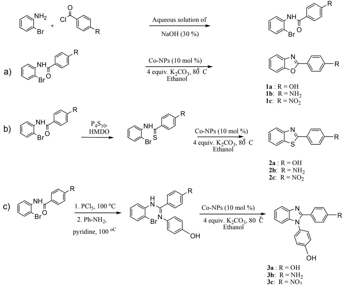
**Scheme 1.** Synthesis of derivatives of benzoxazoles (a), benzothiazoles (b) and benzimidazoles (c), catalyzed by Co-NPs.
