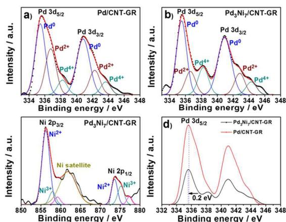
Fig. 4 Pd 3d and Ni 2p XPS spectra; a) Pd in Pd/CNT-GR, b) Pd in Pd<sub>3</sub>Ni<sub>7</sub>/CNT-GR, c) Ni in Pd<sub>3</sub>Ni<sub>7</sub>/CNT-GR, and d) comparison of Pd spectra in Pd/CNT-GR and Pd<sub>3</sub>Ni<sub>7</sub>/CNT-GR.
