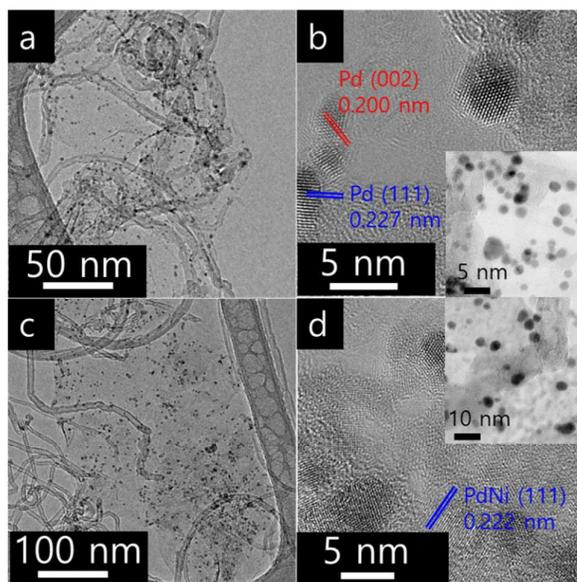
Fig. 2 TEM images of Pd/CNT-GR (a,b) and  $Pd_3Ni_7/CNT-GR$  (c,d).
