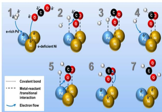
Pure formic acid was successfully produced via CO<sub>2</sub> hydrogenation for the first time over a heterogeneous catalyst of PdNi alloy on carbon na
