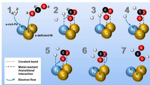
Scheme 1. A proposed reaction mechanism of selective formation of HCOOH from CO<sub>2</sub> hydrogenation over PdNi bimetallic surface. The  $\delta^+/\delta^-$  signs in the illustration represent the localized electron charge in the molecules or bimetallic structure.
