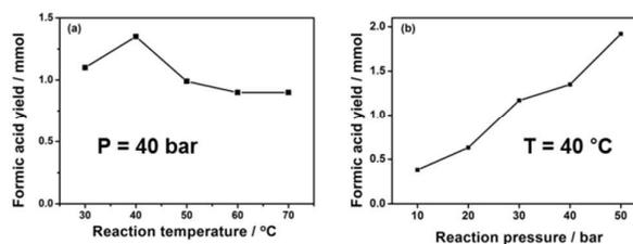
Fig. 6 Formic acid yields as functions of (a) reaction temperature and (b) reaction pressure. Reaction conditions: 1 mmol Pd<sub>3</sub>Ni<sub>7</sub>/CNT-GR, 90 ml H<sub>2</sub>O, H<sub>2</sub>/CO<sub>2</sub> = 1, 15 h.
