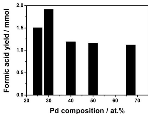
Fig. 5 Formic acid yields as a function of Pd content. Reaction conditions: 1 mmol (Pd+Ni) catalysts, 90 ml H<sub>2</sub>O, P = 50 bar (H<sub>2</sub>/CO<sub>2</sub> = 1), 40 °C, 15 h.
