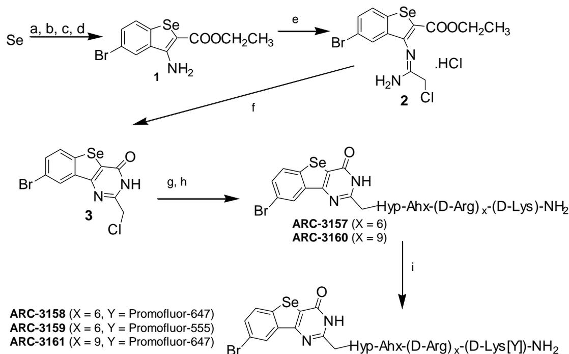
Scheme 1 Synthetic route to ARC-Lum(Fluo) probes: a) NaBH<sub>4</sub>/H<sub>2</sub>O, 0 °C; b) 5-Bromo-2-fluorobenzonitrile, DMF, 0-20 °C; c) BrCH<sub>2</sub>COOCH<sub>2</sub>CH<sub>3</sub>, 0-20 °C; d) 4M NaOH, 0-60 °C; e) chloroacetonitrile, 4N HCl in dioxane; f) dioxane, reflux; g) peptide on resin, DIPEA, 60 °C, 8h; h) TFA, TIS, H<sub>2</sub>O; i) NHS ester of PromoFluor dye, TEA, DMSO.
