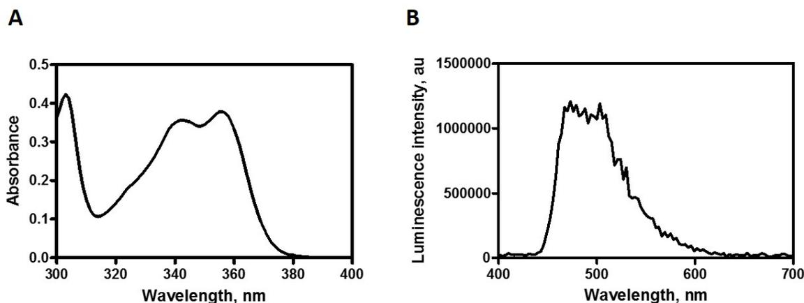
Fig. 3 Optical spectra of an ARC-Lum(-) probe ARC-3157. (A) UV absorption spectrum of ARC-3157 (670  $\mu$ M) in water, pH 7.4 (path length 1 mm). (B) Phosphorescence emission spectrum of ARC-3157 (200 nM) in complex with PIM-2 (200 nM) in assay buffer (50 mM HEPES, 150 mM NaCl, 0.005% Tween 20, 5 mM DTT and 0.5 mg/ml BSA). Excitation at 360(5) nm, delay time 50  $\mu$ s and gate 200  $\mu$ s.
