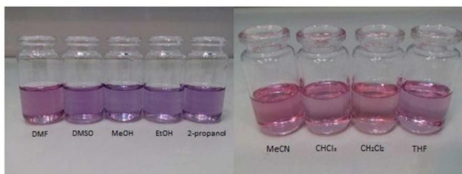
**Figure 1.** Solvatochromic behaviour of 2-amino-3-phenylnaphtho[2,3-*b*]furan-4,9-dione.
