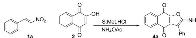
**Scheme 1.** The trial synthesis of 2-amino-3-phenylnaphtho[2,3-*b*]furan-4,9-dione.
