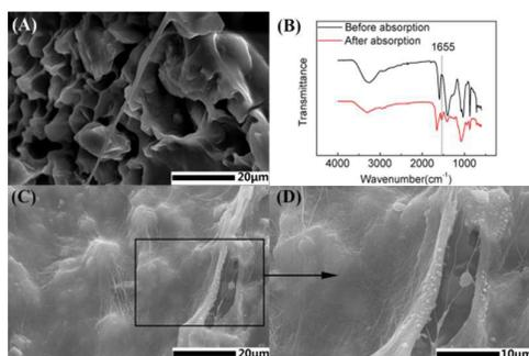
Figure 7 Surface morphology images (A) before and (C, D) after protein absorption; (B) FTIR spectrum of hydrogels
