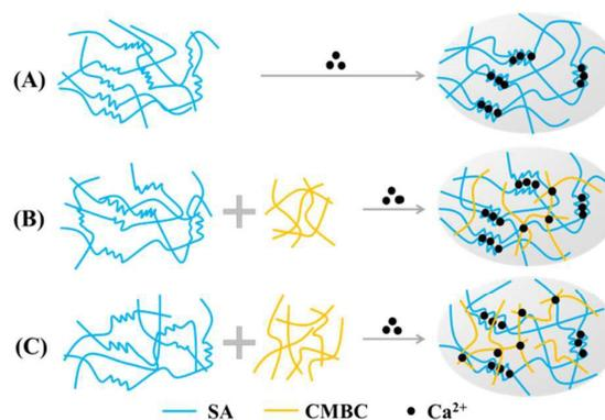
Fig. 2 Cross-linking mechanisms of (A) SA with no CMBC; (B) SA with moderate CMBC; (C) SA with excessive CMBC
