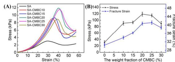
Figure 4 (A) Stress-strain curve of series of SA/CMBC composites; (B) Mechanical property with different weight fraction of CMBC
