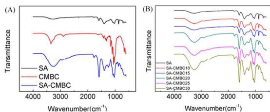
Fig. 3 (A) Infrared spectroscopy curves of SA, CMBC and SA-CMBC; (B) Infrared spectroscopy curves of gels with different weight fractions of CMBC
