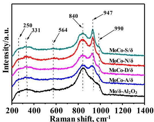
Fig. 4. Raman spectra of the MoCo/ $\delta$  catalysts with different cobalt salts.
