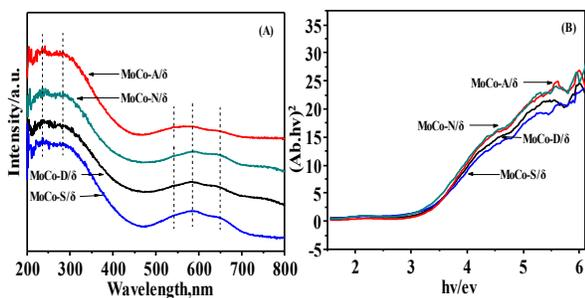
Fig. 2. (A) UV-vis DRS spectra, (B) plots of a  $1/2$  versus photon energy ( $h\nu$ ) of MoCo/ $\delta$  with different cobalt salts.
