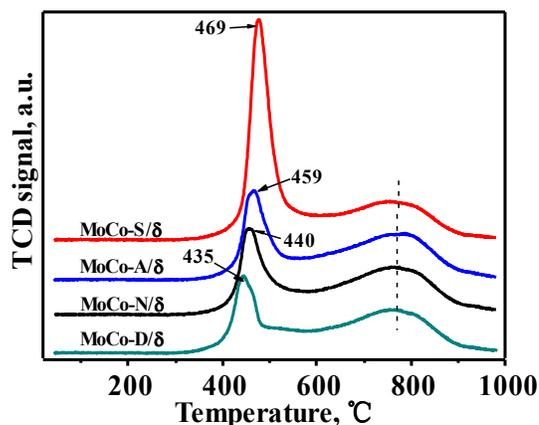
Fig. 3. H<sub>2</sub>-TPR profiles of MoCo/ $\delta$ -Al<sub>2</sub>O<sub>3</sub> with different cobalt salts.
