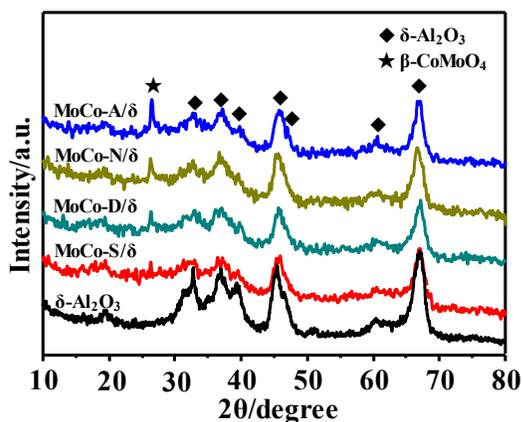
Fig. 1. XRD patterns of the series supports and catalysts with different cobalt salts.
