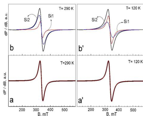
**Figure 13.** EPR spectra at 290 and 120 K of NMP/C electrode before the electrochemical reaction (a, a'); NMP/C electrode after 5 cycles between 2.5 and 4.5 V (b, b'). The black curves are the experimental EPR spectra, while the red and blue curves correspond to the deconvoluted signal 1 and signal 2.
