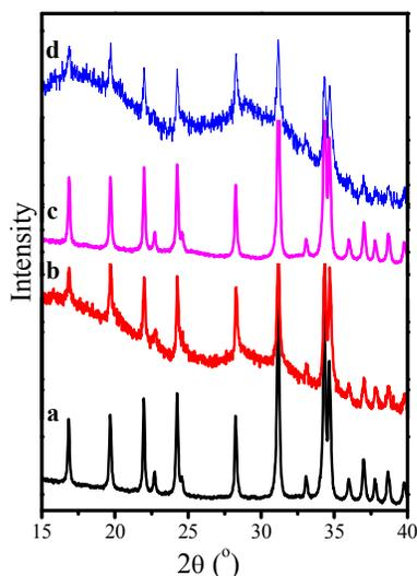
**Figure 6.** XRD patterns of: (a) pristine NMP; (b) pristine NMP after soaking in the lithium electrolyte; (c) NMP/C composite; and (d) NMP/C after soaking in the electrolyte.
