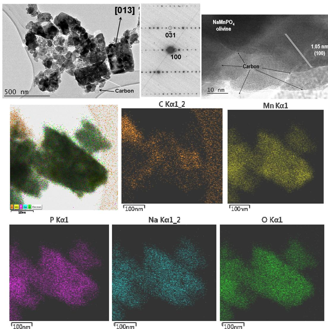
**Figure 5.** Bright field micrographs and SAED of composite NMP/C (left, first row); HRTEM image (right, first row); BF-STEM images and corresponding composition map of  $\text{CK}\alpha_{1-2}$ ,  $\text{MnK}\alpha_1$ ,  $\text{PK}\alpha_1$ ,  $\text{NaK}\alpha_{1-2}$  and  $\text{OK}\alpha_1$ .
