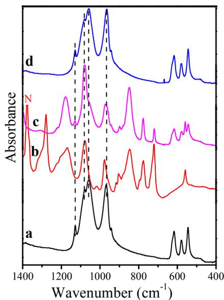
**Figure 7.** IR spectra of NMP/C composite (a), fresh electrolyte LiPF<sub>6</sub> in EC/DMC (b), NMP/C after soaking in the lithium electrolyte (c); NMP/C after soaking in the lithium electrolyte and washed with acetone (d). "N" denotes the band from Nujol oil.
