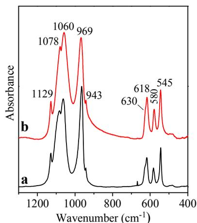
**Figure 2.** IR spectra of pristine NMP (a) and NMP/C composite (b).
