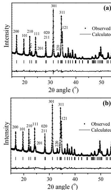
**Figure 1.** Rietveld refinement of the XRD patterns of pristine NaMnPO<sub>4</sub> (a) and NaMnPO<sub>4</sub>/C composite (b).
