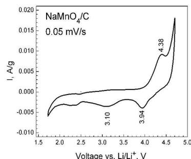
**Figure 9.** CV curve of  $\text{NaMnPO}_4/\text{C}$  in a lithium cell after 5 galvanostatic cycles between 2.5 and 4.5 V.
