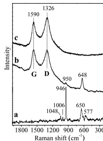
**Figure 3.** Raman spectra of NMP (a), NMP/C (b) and carbon additives (c).
