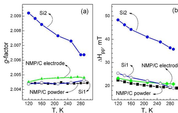
**Figure 14.** Temperature dependence of the *g*-factor (a) and EPR line width (b) for NMP/C powder (square symbols), NMP/C electrode before the electrochemical reaction (triangular symbols) and NMP/C electrode after 5 cycles between 2.5 and 4.5 V at C/50 (open and full circles for Si1 and Si2).
