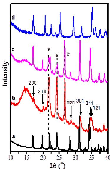
**Figure 10.** XRD patterns of NMP/C composite (a), NMP/C after 5 charge-discharge cycles between 4.5 and 2.5V at C/50 (b), NMP/C electrode prior to cycling (c) and  $\text{LiMnPO}_4$  (d). Symbols “P” and “C” denote the diffraction peaks due to parafilm and graphite.
