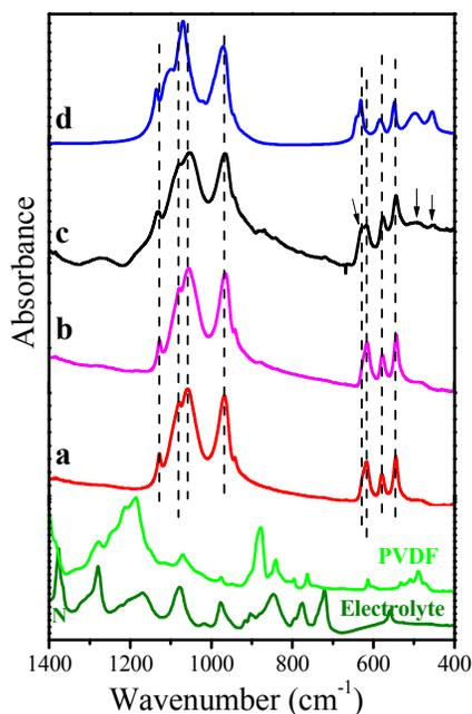
**Figure 12.** IR spectra of NMP/C composite (a), NMP/C electrode prior to electrochemical reaction (b), NMP/C electrode after 5 charging-discharging cycles between 4.5 and 2.5V at C/50 (c), LiMnPO<sub>4</sub> reference (d). For the sake of comparison, PVDF and electrolyte LiPF<sub>6</sub>/EC/DMC are also given.
