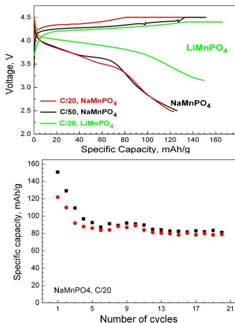
**Figure 8.** First charging/discharging curves for  $\text{NaMnPO}_4$  and  $\text{LiMnPO}_4$  used as electrodes in model lithium cells. The charge and discharge capacity (black and red symbols) for  $\text{NaMnPO}_4$  versus the number of cycles.
