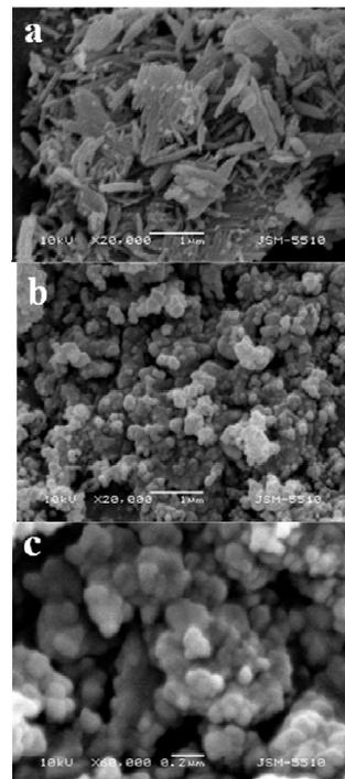
**Figure 4.** SEM images of pristine NMP (a) and NMP/C composite (b). For NMP/C, a higher magnification is used (c).
