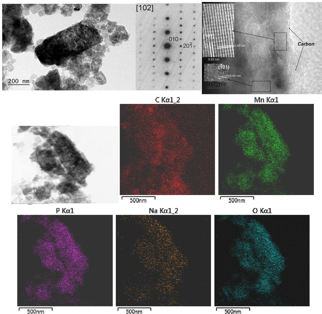
**Figure 11.** *ex-situ* Bright field micrographs and SAED of NMP/C electrode cycled 5 times between 2.5 and 4.5 V at C/50 in a model lithium cell (left, first row); HRTEM image (right, first row); BF-STEM images and corresponding composition map of  $CK\alpha_{1,2}$ ,  $MnK\alpha_1$ ,  $PK\alpha_1$ ,  $NaK\alpha_{1,2}$  and  $OK\alpha_1$ .
