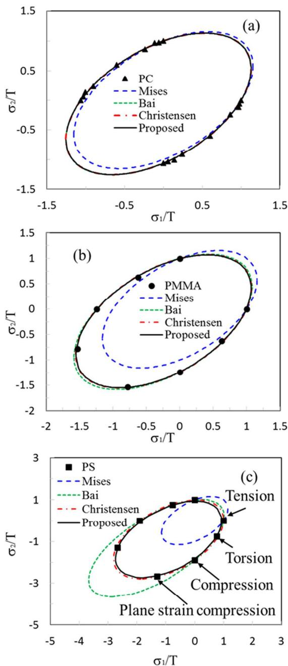
**Fig.2** Comparison between the experiment data with four forms of equivalent stress in plane stress space, i.e., Mises, Bai, Christensen and the proposed form: (a) PC, (b) PMMA (@60°C), (c) PS (@90°C). The experiment data of PMMA and PS are from the literature.<sup>27</sup>
