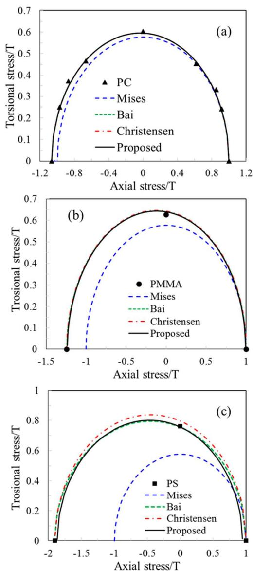
**Fig.1** Comparison between the experiment data with four forms of equivalent stress under combined axial-torsional condition, i.e., Mises, Bai, Christensen and the proposed form: (a) PC, (b) PMMA (@60°C), (c) PS (@90°C). The experiment data of PMMA and PS are from the literature.<sup>27</sup>
