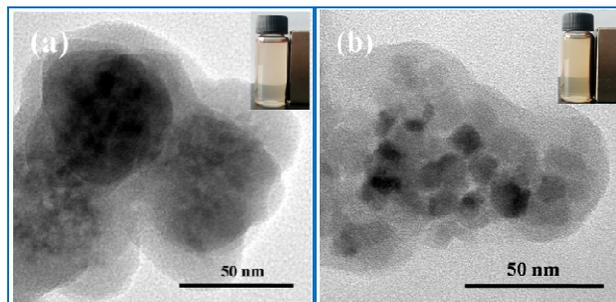
Fig. 4 TEM images of (a) MSNPs and (b) AF-MSNPs. The inserts are the magnetic performance of the magnetic carriers.
