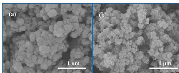
Fig. 3 SEM images of (a) MSNPs and (b) AF-MSNPs.
