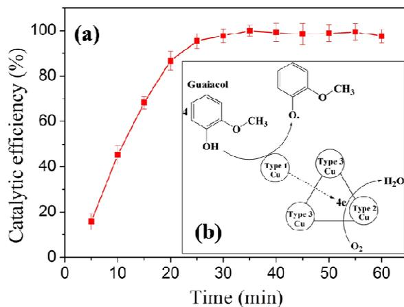
Fig. 10 Catalytic efficiency of guaiacol by immobilized laccase. (a) The curves of the catalytic efficiency as a function of time; (b) The mechanism of catalytic the guaiacol by immobilized laccase
