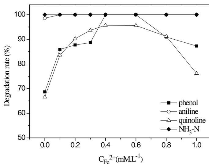
Fig. 6. Effect of Fe(II) concentration on pollutants degradation in the  $\text{O}_3$ /Fenton process.
