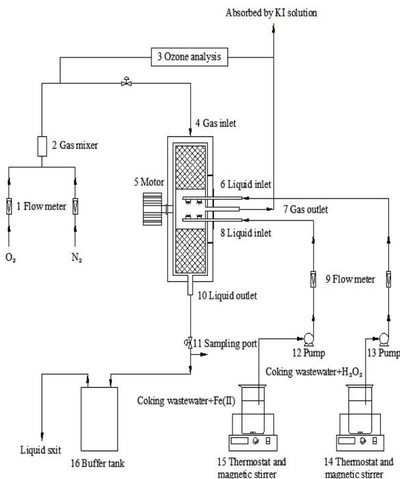
Fig. 1. Experimental setup for the treatment of simulated coking wastewater in an RPB with the  $\text{O}_3/\text{Fenton}$  process.
