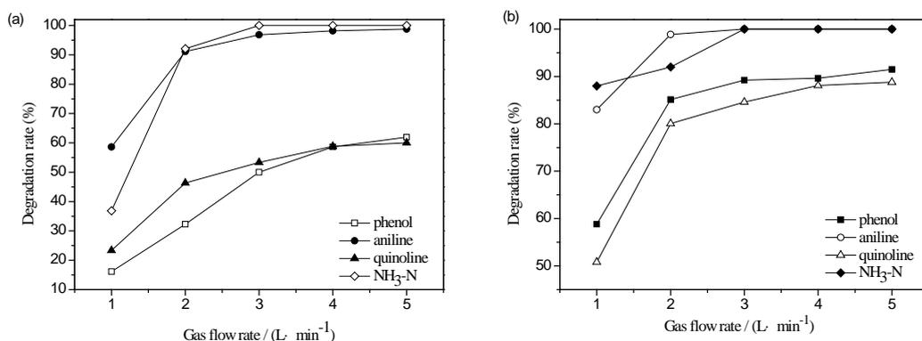
Fig. 3. Effect of gas flow rate on pollutants degradation in the O<sub>3</sub> process (a) and O<sub>3</sub>/Fenton process (b).
