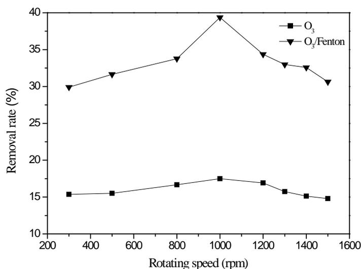
Fig. 2. Effect of rotation speed on the COD removal rate.
