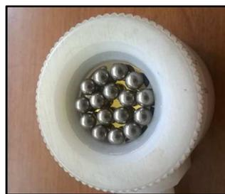
Fig. 2. Photograph of the QCM holder held horizontally with sixteen ball bearings loaded onto its surface electrode.
