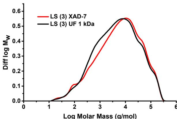
**Fig. 7** Molecular weight distribution of lignosulfonates isolated by preparative-scale XAD-7 method and UF 1kDa.
