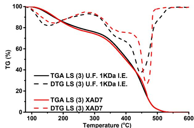
**Fig.8** Thermogravimetry (TG) and differential thermogravimetry (DTG) curves of lignosulfonate purified by XAD-7 adsorption and ultrafiltration techniques.
