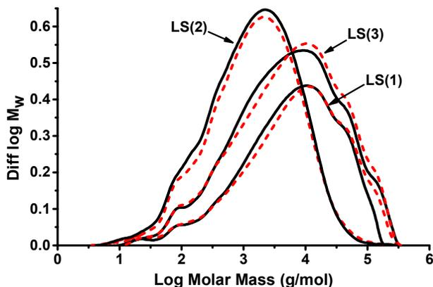
**Figure 6.** MMD of two isolations performed in parallel (dashed and solid curves) by preparative-scale XAD-7 for three lignosulfonates samples.
