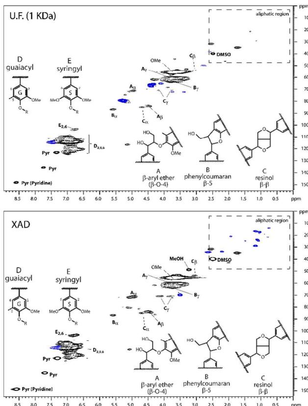
Fig. 9 Comparison of HSQC NMR spectra (acquired in DMSO/pyridine) of lignosulfonate samples purified by ultrafiltration through a 1 kDa membrane (top) and XAD-7 adsorption (bottom). Blue coloured peaks highlight major differences in the samples, the colour code having been introduced post processing.
