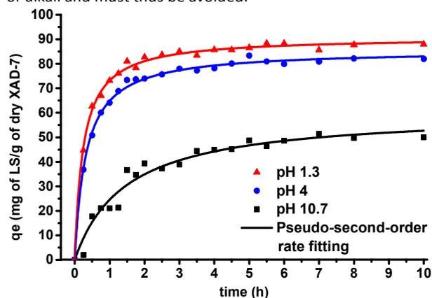
**Fig. 1** The effect of pH on the adsorption of lignosulfonates on XAD-7 resin (adsorbate/adsorbent proportion:  $130 \text{ mg g}^{-1}$ ) at  $25^\circ \text{C}$ .
