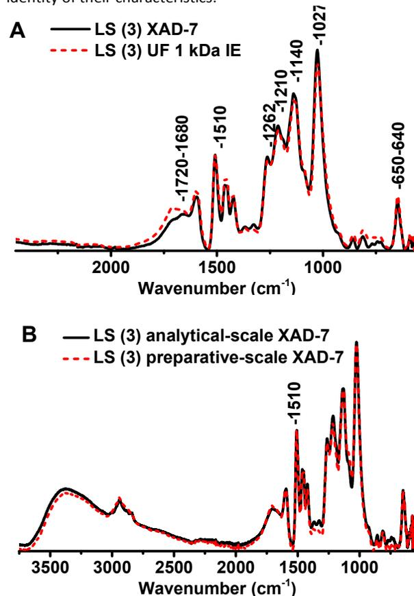
**Fig. 5** A: FTIR spectra of Liginosulfonate (3) isolated by ultrafiltration (after cation exchange) and XAD-7 adsorption. B: FTIR spectra of the same Liginosulfonate (3) isolated by analytical and preparative XAD-7 adsorption
