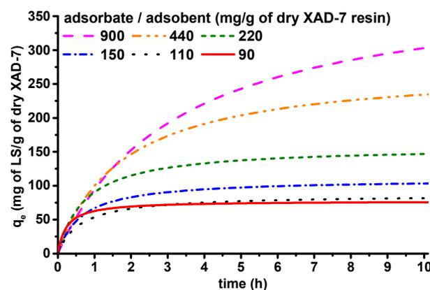
**Fig. 2** The adsorption kinetic for the uptake of lignosulfonates onto XAD-7 resin at different adsorbate/adsorbent proportion at pH 2 and  $25^\circ \text{C}$ .
