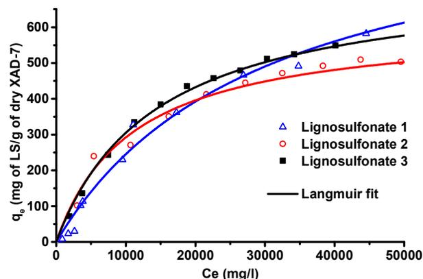
**Fig. 3** Isotherm models of lignosulfonate (1-3) adsorption by XAD-7 resin at pH 2 and 25 °C.
