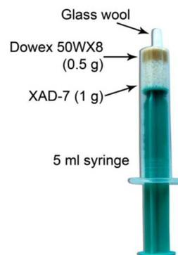
**Fig. 4** Syringe filled with resins used for fast analytical-scale XAD-7 adsorption of lignosulfonates.
