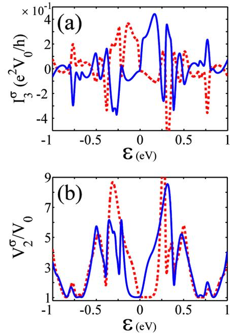
FIG. 4: (Color online) (a) The fully spin-polarized currents in terminal 3 and (b) the ratio of voltages  $V_2^{\sigma}(\varepsilon)/V_0$  as a function of electron energy. The solid (blue) and dashed (red) curves correspond to spin-up and spin-down electrons, respectively.
