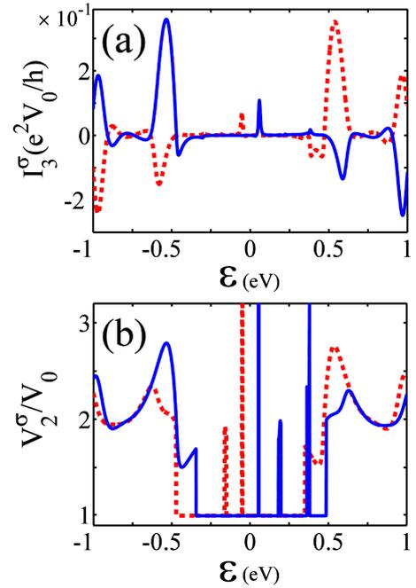
FIG. 2: (Color online) (a) The fully spin-polarized currents in terminal 3 and (b) the ratio of voltages  $V_2^\sigma/V_0$  as a function of electron energy. The solid (blue) and dashed (red) curves correspond to spin-up and spin-down electrons, respectively.
