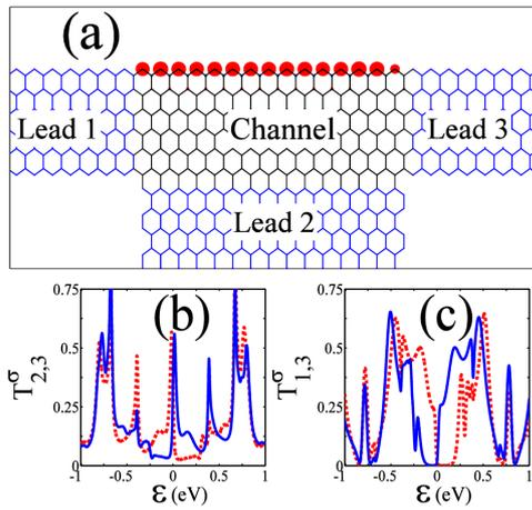
FIG. 3: (a) Schematic view of a three-terminal T-shaped junction with localized magnetic moments at zigzag edge; the red circles correspond to the majority spin electrons. (b) and (c) show the spin and energy-dependent transmission coefficient between the drain 1 and drain 2 and between source and drain 2, respectively. The solid (blue) and dashed (red) curves correspond to spin-up and spin-down electrons.
