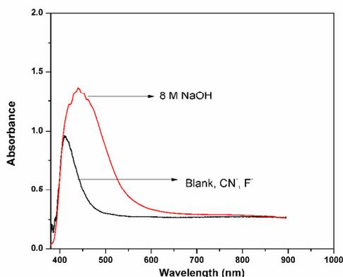
Fig. 5 Absorbance spectra of the optode in the presence of cyanide and fluoride ions (8M) and 8 M hydroxide ions
