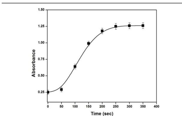
Fig. 4 Absorbance as a function of equilibration time of the sample in 10 mL of 8 M hydroxide solution
