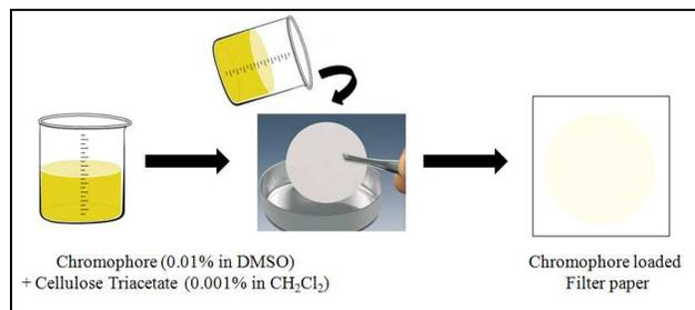
Scheme2. Pictorial representation of the fabrication steps of sensor strip
