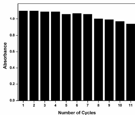
Fig. 6 Absorbance of the same optode strip over 12 cycles of measurement
