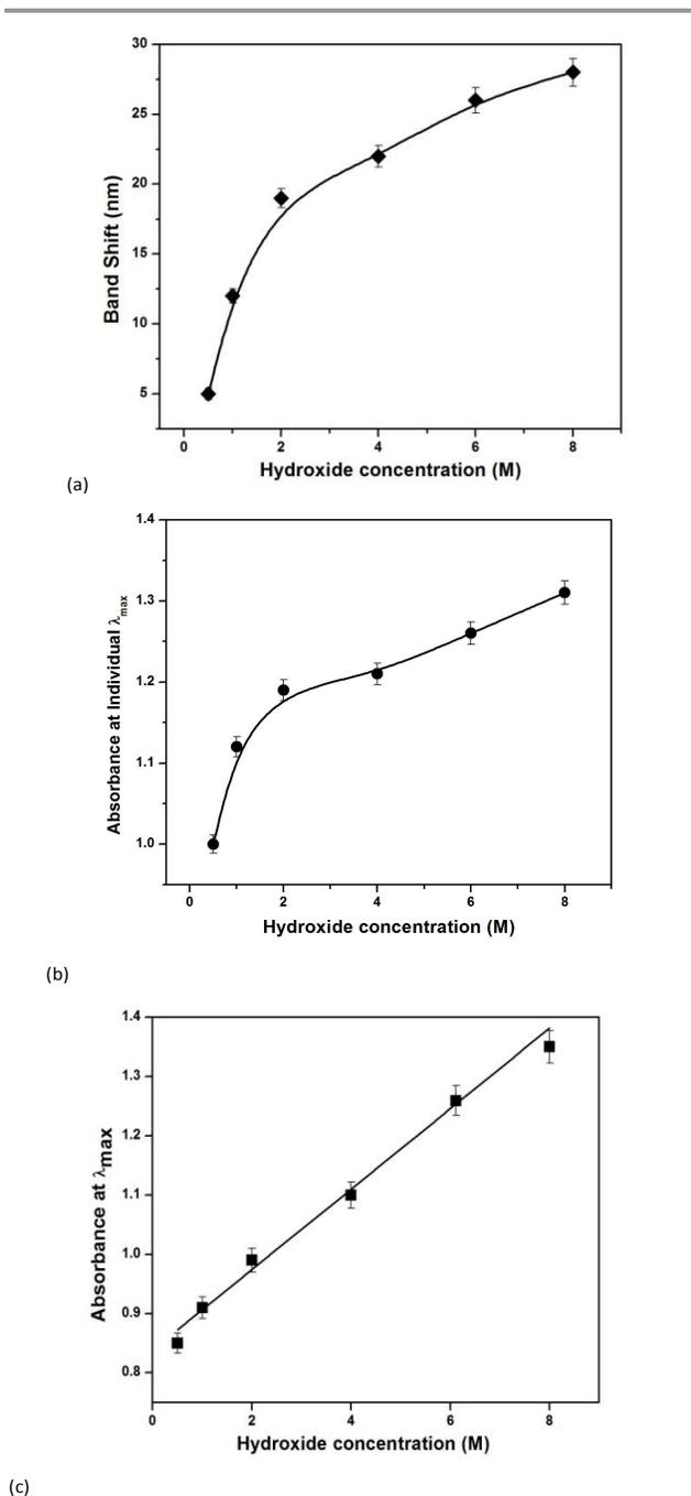
Fig. 3 Variations of absorbance at  $\lambda_{\max}$  shift (spectral shift) (a)  $\lambda_{\max}$  (b), and absorbance at 438.1 nm (c) as a function of hydroxide concentration of from 0.5 M to 8 M
