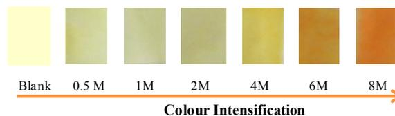
Fig. 7 Change in the color of strip sensor with varying concentration of hydroxide ions
