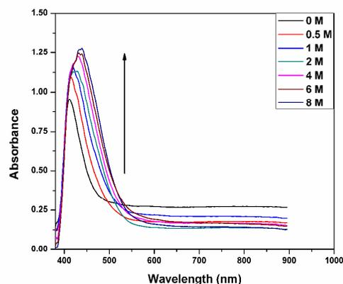
Fig. 2 Absorbance spectra of the sensor strip equilibrated with 0.5 M to 8 M hydroxide solution
