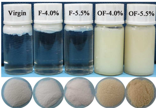
Figure 1. Photograph of dispersibility of UHMWPE particles in deionized water.
