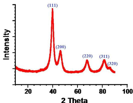
Fig. 1. XRD of Md-Pt NPs@AC.
