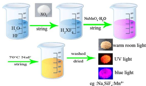
**Fig. 1** Schematic diagram of the preparation process for NXFM phosphors *via* chemical co-precipitation method.
