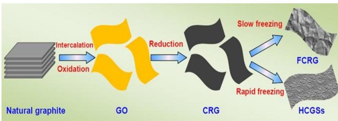
**Fig. 19:** schematically describes the whole synthetic procedure for the fabrication of HCGSs [52]. Copyright 2013, The Royal Society of Chemistry
