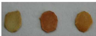
Figure 7 Change in color of PITP absorbed on paper upon adding buffer solutions (containing 60% methanol) at pH- 7.5, 4.2, 2.0 (left to right).
