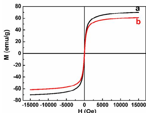
**Fig. 2** Magnetization curves of Fe<sub>3</sub>O<sub>4</sub> nanoparticles (a) and MPS-Fe<sub>3</sub>O<sub>4</sub> nanoparticles (b).
