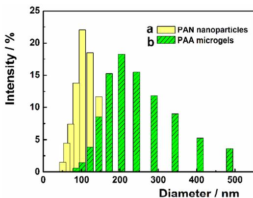
Fig. 7 Size distributions of PAN nanoparticles and PAA nanogels.
