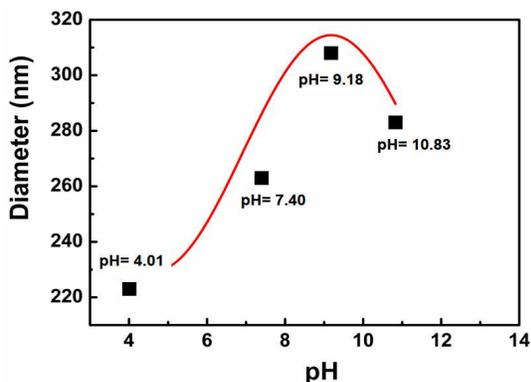
Fig. 8 pH-responsive property of PAA nanogels at pH (a) 4.01, (b) 7.40, (c) 9.18, and (d) 10.83, respectively.
