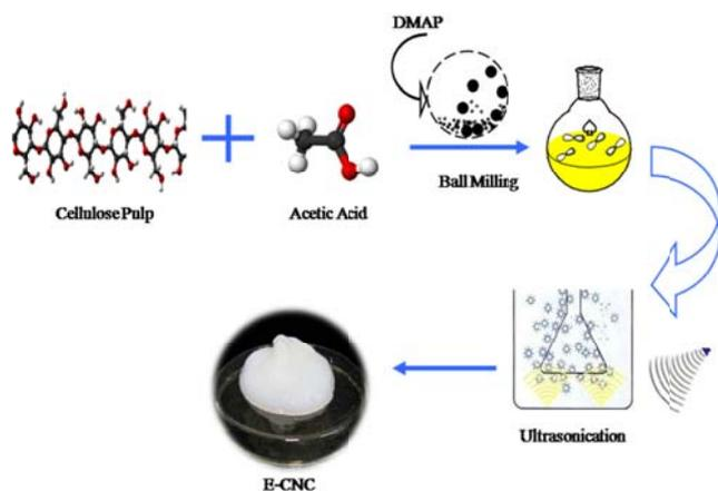
Fig. 1 Schematic model of the manufacture of E-CNC via one-pot tandem reactions.
