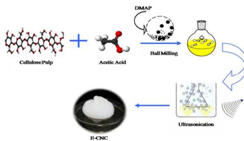
Esterified cellulose nanocrystals were manufactured via one-pot tandem reactions with DMAP as catalyst, during the process cellulose nanocrystallization and acetylation occurred simultaneously.
