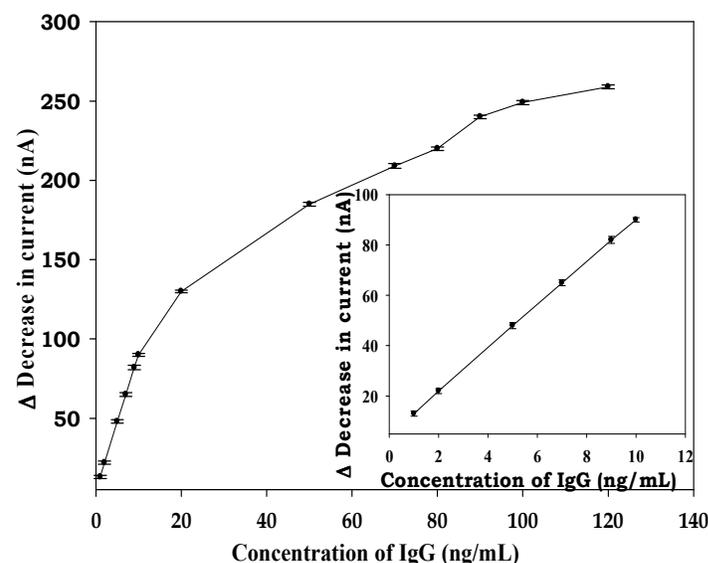
**Fig. 4 (b).** Calibration plot of decrease in DPV peak current vs mouse IgG concentration ( $n=3$ ). Inset shows linear calibration curve at lower range (1.0 to 10.0 ng/mL).
