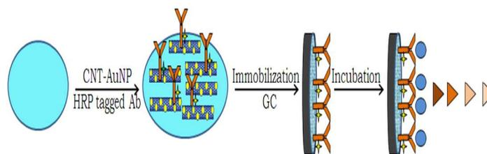
Scheme 1 Schematic representation of fabrication of immunosensor
