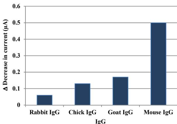
**Fig. 5.** Bar graph of decrease in DPV peak current response vs specificity of the immunosensor after interaction with different antigens of same concentration  $0.1\mu\text{g/ml}$  (a) mouse IgG, (b) chicken IgG, (c) rabbit IgG and (d) goat IgG
