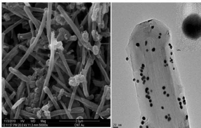
**Fig 1(a)** SEM image and **(b)** TEM image of CNT-AuNPs hybrid nanocomposite (inset shows the single AuNP).
