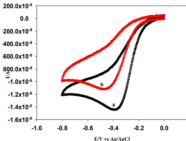
**Fig 3.** Cyclic voltammograms in 0.1 M phosphate buffer (pH 7.4) 0.1 M KCl at 10 mV/s of different modified GC electrode: nafion/CNT-AuNPs and HRP tagged rabbit antimouse IgG (nafion/CNT-AuNPs/Ab-HRP) on GC electrode without incubation with mouse IgG antigen (curve a), and after interaction with mouse IgG 0.5  $\mu\text{g/mL}$  on CNT-AuNPs and HRP tagged rabbit antimouse IgG modified GC electrode (curve b).
