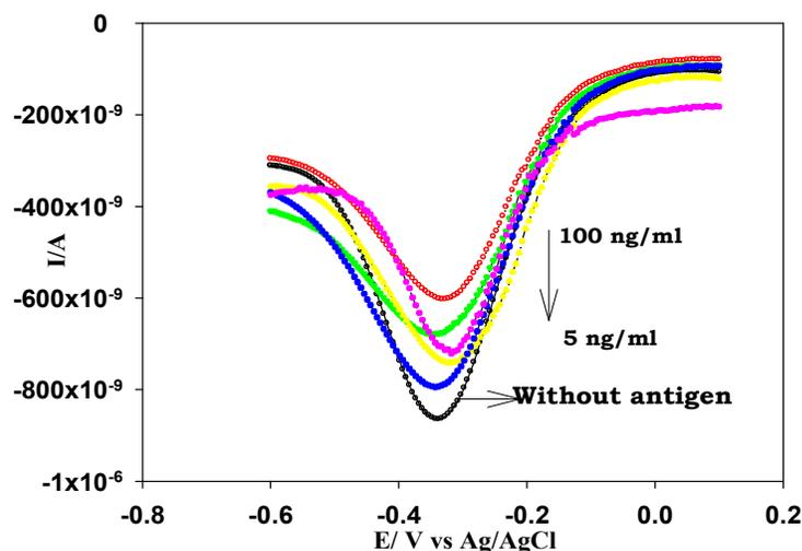
**Fig. 4 (a)** DPV of the immunosensor in 0.1 M phosphate buffer (pH 7.4) 0.1 M KCl after interaction with different concentrations of mouse IgG.
