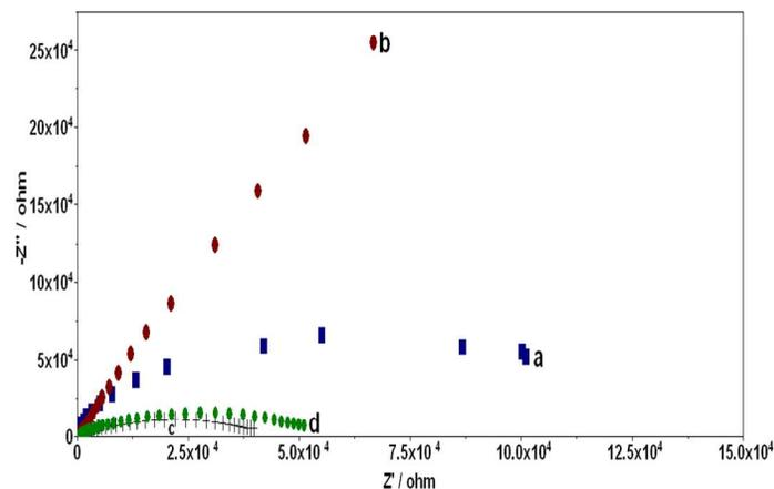
**Fig 2** Nyquist plot in 1.0 mM Fe(CN)<sub>6</sub><sup>-3/4-</sup> containing 0.1 M KCl of different modified GC electrode (a) nafion modified GC electrode, (b) nafion/CNT-AuNPs on GC electrode, (c) nafion/CNT-AuNPs and HRP tagged rabbit antimouse IgG (nafion/CNT-AuNPs/Ab-HRP), (d) Immunoconjugate is formed after interaction with mouse IgG on CNT-AuNPs and HRP tagged rabbit antimouse IgG modified GC electrode.
