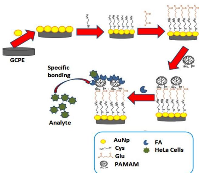
**Scheme 1.** Schematic illustration of step by step preparation of the GCPE/AuNP/Cys/Glu/Pamam/FA cytosensor.
