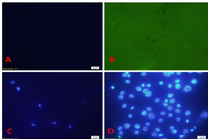
**Figure 2.** Fluorescence microscopy image of **A)** bare ITO electrode, **B)** FA/PAMAM/Glu/Cys/AuNp/ITO modified electrode, **C)** A549/FA/PAMAM/Glu/Cys/AuNp/ITO electrode and **D)** HeLa/FA/PAMAM/Glu/Cys/AuNp/ITO electrode. [Image B was obtained under the green filter for monitoring the fluorescence of AuNps and Image C and D were obtained under the blue filter for monitoring the DAPI treated samples (Scale of the each image was 10  $\mu\text{m}$ ).]
