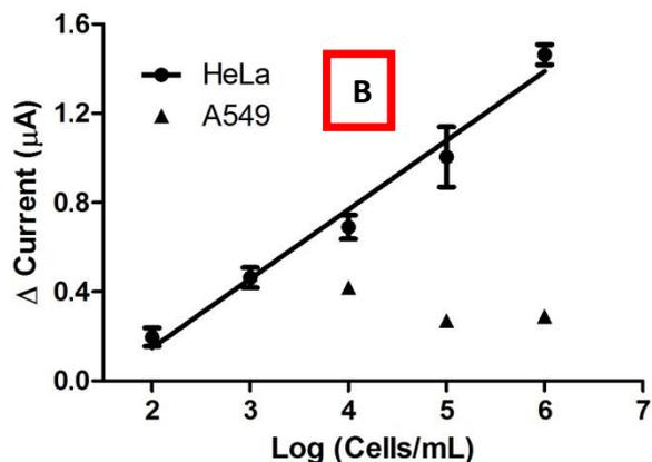
**Figure 5. A)** CV voltammograms for the linear range. (a)  $10^6$ , (b)  $10^5$ , (c)  $10^4$ , (d)  $10^3$  and (e)  $10^2$  cells/mL. **B)** Calibration graph was obtained for HeLa and A549 cells with GCPE/AuNp/Cys/Glu/Pamam/FA cytosensor under optimized parameters (25 mM FA, 60 min). These measurements were performed in 50 mM PBS pH 7.0, temperature of 25°C, working potential 0.4 V to -0.1 V and scan rate 0.05 v/s.
