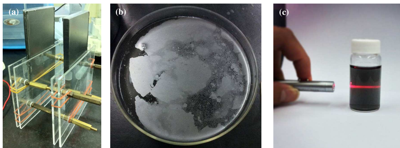
Figure 1. (a) Experimental set-up of electrochemical exfoliation system; (b) Silver-like substances floated on the electrolyte solution. (c) Highly dispersion of EC-graphene suspension with Tyndall effect were obtained after exfoliation process.
