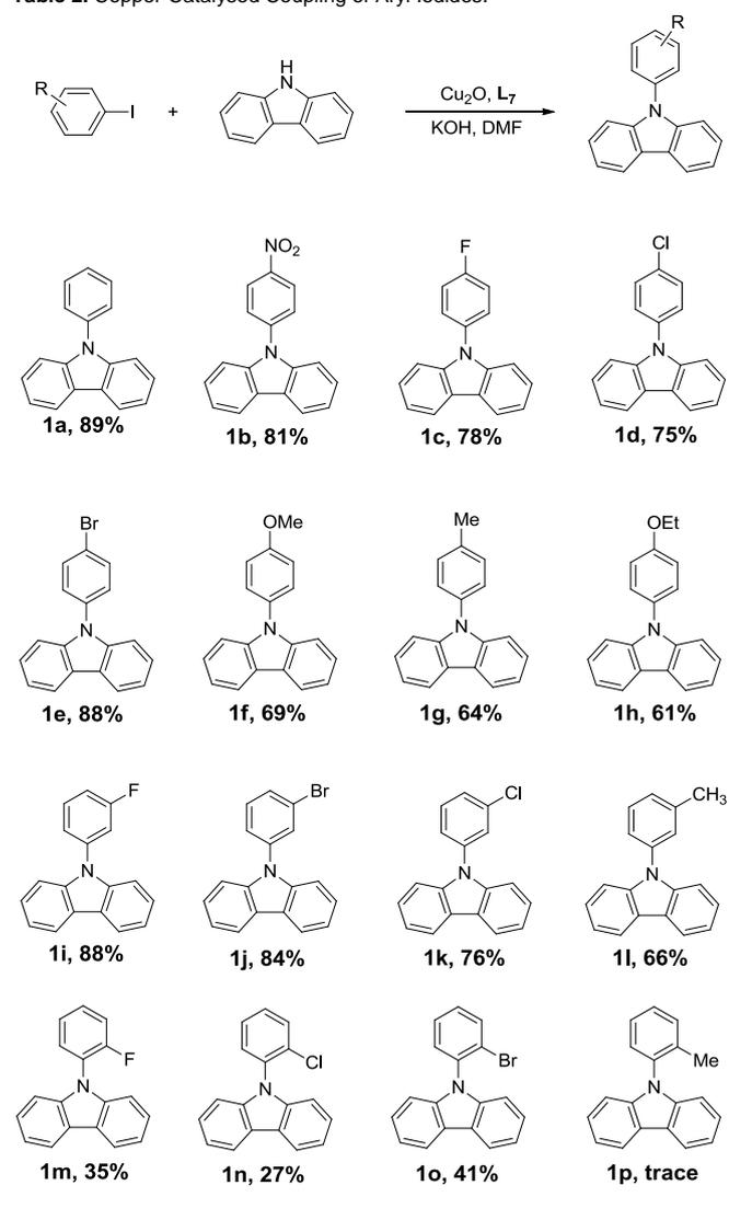
[a] Reaction conditions: Aryl iodides (0.5 mmol), Carbazole (0.75 mmol), Cu<sub>2</sub>O (10 mol%), L<sub>7</sub> (10 mol%), KOH (1.0 mmol) in DMF (2 mL) under N<sub>2</sub>, 110 °C, 24 h. Isolated yield.
