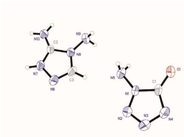
**Figure 9.** View of the molecular unit of 3,4-diamino-1,2,4-triazolium 1-aminotetrazol-5-oneate (**7f**) with thermal ellipsoids at the 50% probability level. Selected bond distances and angles in the anion of **7f**: bond lengths [Å] N(6)-C(3) 1.279(5), N(6)-N(7) 1.393(4), N(7)-C(2) 1.311(5), N(8)-C(2) 1.363(5), N(8)-C(3) 1.370(5), N(8)-N(9) 1.398(4), N(10)-C(2) 1.296(5); angles [deg] N(10)-C(2)-N(7) 130.3(3), N(10)-C(2)-N(8) 124.9(3), N(7)-C(2)-N(8)
