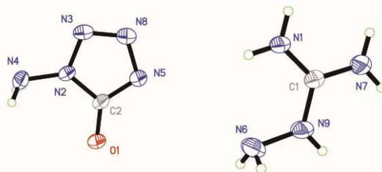
**Figure 6.** View of the molecular unit of aminoguanidinium 1-aminotetrazol-5-oneate (**7c**) with thermal ellipsoids at the 50% probability level. Selected bond distances and angles in the anion of **7c**: bond lengths [Å] C(1)-N(1) 1.3169(13), C(1)-N(9) 1.3266(14), C(1)-N(7), 1.3317(14), N(6)-N(9) 1.4046(15); angles [deg] N(1)-C(1)-N(9) 120.54(10), N(1)-C(1)-N(7) 121.67(10), N(9)-C(1)-N(7) 117.79(10), C(1)-N(9)-N(6) 119.22(10).
