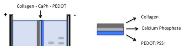
**Figure 2.** Formation of a PEDOT:PSS layer over collagen-calcium phosphate membrane. After the formation of collagen-calcium phosphate, PEDOT:PSS is added in the electrolyte and its active potential (-1.2 V vs. Pt) is applied for 1800 s. As a result, PEDOT:PSS forms a layer over the collagen-calcium phosphate.
