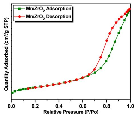
Figure 1: BET surface of Mn/ZrO<sub>2</sub> catalyst
