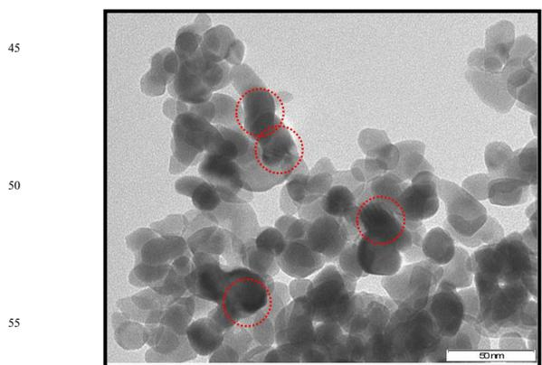
Figure 5. TEM image of Mn/ZrO<sub>2</sub> catalyst
