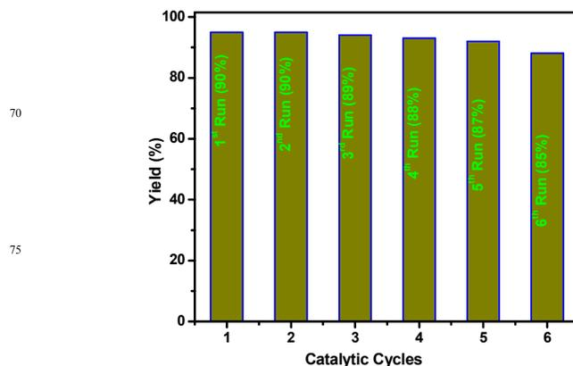
Figure 6. Recyclability of Mn/ZrO<sub>2</sub> catalyst
