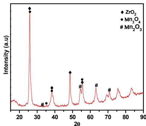
Figure 2. Powder X-ray diffractogram spectra of Mn/ZrO<sub>2</sub> catalyst
