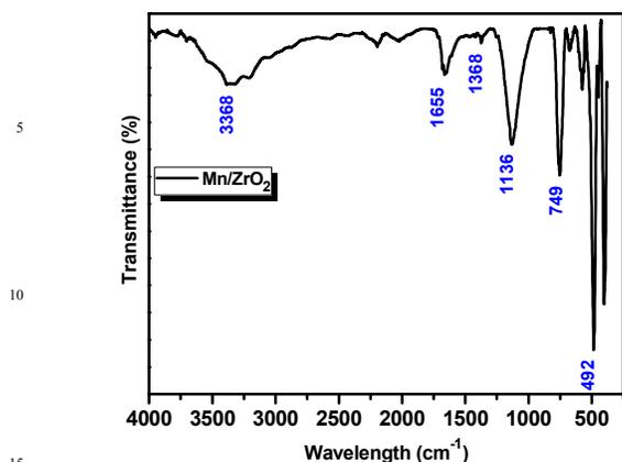
Figure 3. FT-IR image of Mn/ZrO<sub>2</sub> catalyst
